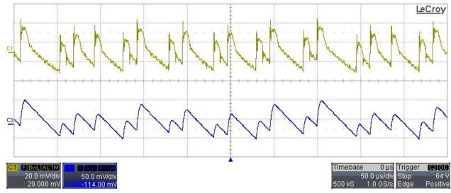
Ch1: 3.3Vout (20mV/div, 20MHz BWL, AC coupling, 50usec/div) Ch2: 12Vout (50mV/div, 20MHz BWL, AC coupling) Vin = 322Vdc
