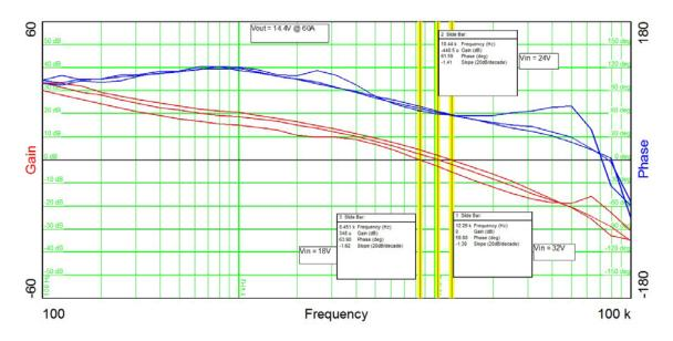
The plot below shows the TPS54060 5V bias supply loop gain for input voltage of 18V and 32V. The output was loaded to 0.5A.
