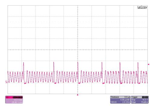
The photo below shows the TPS54060 5V bias supply FET switching voltages (TP5) for an input voltage of 18V and with a 0.5A external load. (10V/DIV, 1uS/DIV)
