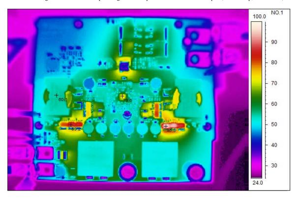
A thermal image is shown below operating at 24V input and 14.4V@30A output (room temp, no airflow).
