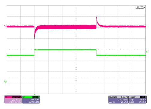
The photo below shows the 14.4V output voltage (ac coupled) when the load current is stepped between 40A and 60A. Vin = 24V. (500mV/DIV, 20A/DIV, 2mS/DIV)
