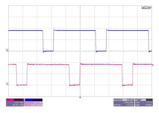
The photo below shows the FET switching voltages (TP15 and TP16) for an input voltage of 18V and a 60A load. (10V/DIV, 2uS/DIV)
