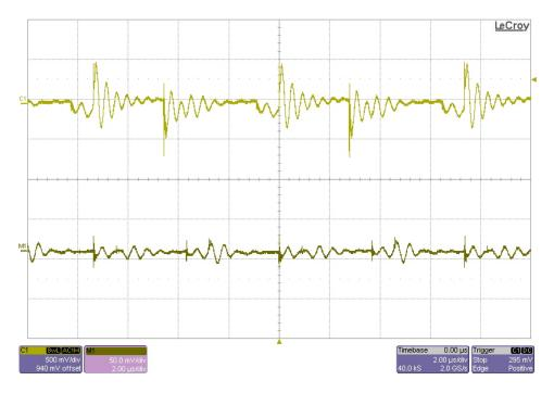
The input ripple voltage (AC coupled) is shown in the figure below. The bottom waveform is measured at the modules input terminals while the top waveform is measured across C26 (after the EMI filter). The image was taken with the output loaded to 60A. The input voltage is set to 18V. (top is 500mV/DIV, bot is 50mV/DIV, 2uS/DIV)
