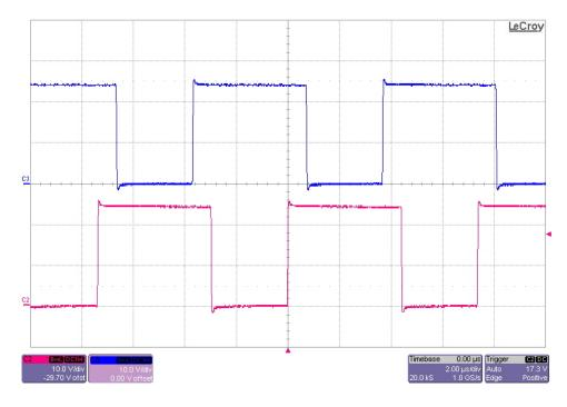
The photo below shows the FET switching voltages (TP15 and TP16) for an input voltage of 24V and a  $60A \log . (10V/DIV, 2uS/DIV)$
