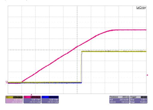
The photo below shows the output voltage startup waveform after the application of 24V in. The 14.4V output was loaded to 0A. RED is Vreg point (TP17), BLUE is Vout (TP19) (5V/DIV, 200mS/DIV)
