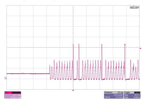
The photo below shows the TPS54060 5V bias supply FET switching voltages (TP5) for an input voltage of 32V and with a 0.5A external load. (10V/DIV, 1uS/DIV)
