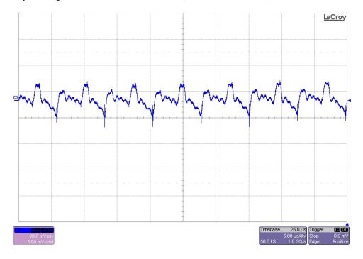
The 14.4V output ripple voltage (AC coupled) is shown in the figure below. The voltage is measured at the modules output terminals. The image was taken with the output loaded to 60A. The input voltage is set to 24V. (20mV/DIV, 5uS/DIV)
