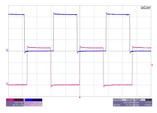
The photo below shows the FET switching voltages (TP15 and TP16) for an input voltage of 32V and a 60A load. (10V/DIV, 2uS/DIV)
