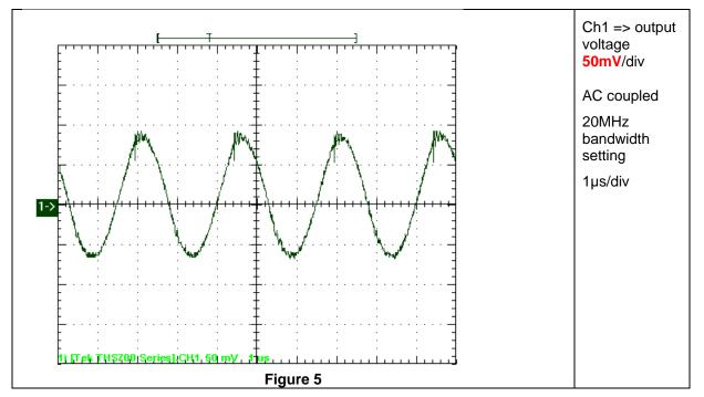
The output ripple voltage before filtering is shown in Figure 6. The image was taken with a 3A load 35V at the input, du 1500mV, filter attenuation 0.1 means -20dB:
