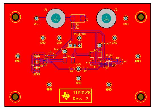
Figure 8: PCB Layout for TIPD178
