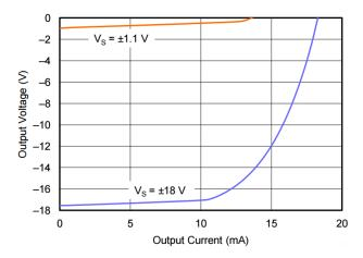
Figure 3: TLV1702 Output Voltage vs. Output Current
