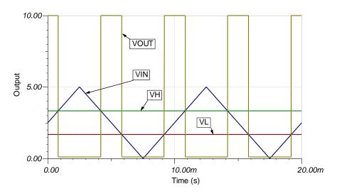
Figure 5: Window Comparator Functionality
