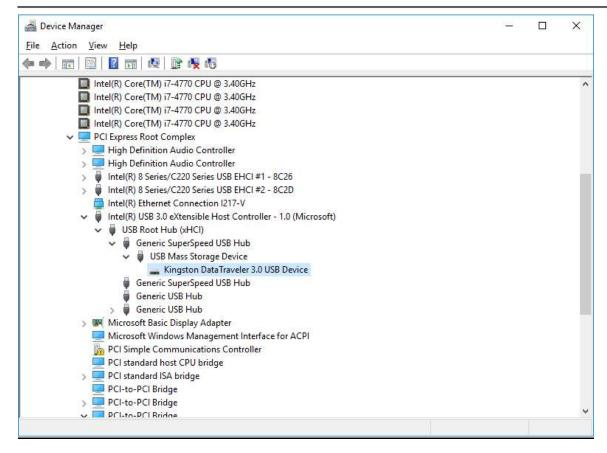
Figure 2 Checking USB connection on Device Manager.
