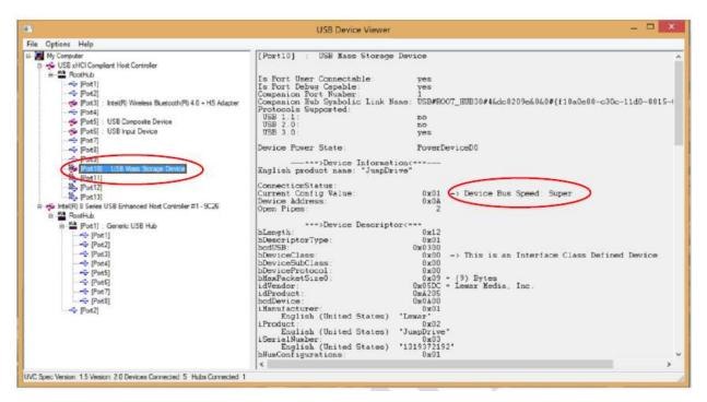
Figure 1 Checking USB connection Speed using USBVIEW
