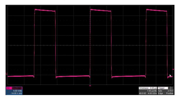
The photo below shows the switch node voltage (TP4). The input voltage is 19V and the 12V output is loaded to 8A. (5V/DIV, 1uS/DIV)
