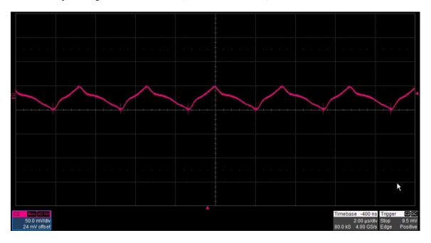
The output ripple voltage is shown in the figure below. The image was taken with the 12V output loaded to 8A and the input voltage set to 24V. (50mV/DIV, 2uS/DIV)
