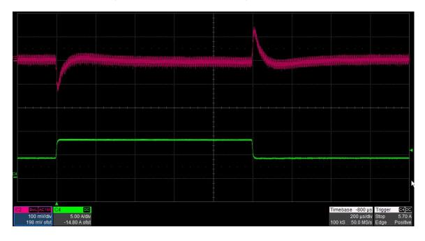
The photo below shows the output voltage (ac coupled) when the load current is stepped between 0A and 8A. Vin = 24V. (200mV/DIV, 5A/DIV, 200uS/DIV)
