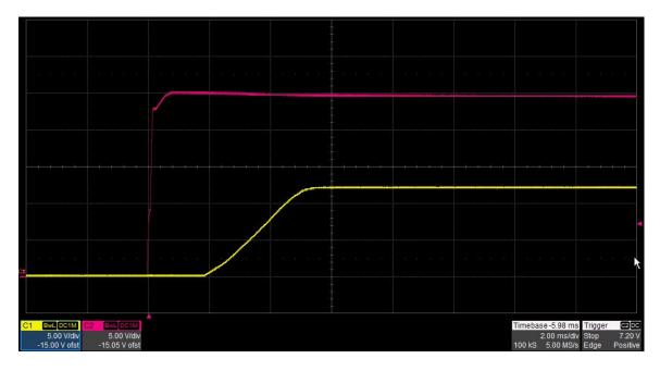
The photo below shows the output voltage startup waveform after the application of 24V in with the 12V output loaded to 8A. (5V/DIV, 2mS/DIV)
