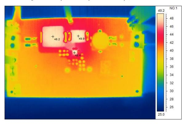
The thermal image below shows operation at 5V input and 15V@1.5A output, with no airflow.
