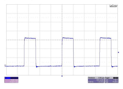
The photo below shows the switch node voltage. The input voltage is 5V and the 15V output is loaded to 80mA. The converter has entered Discontinuous Conduction Mode. (5V/DIV, 500nS/DIV)
