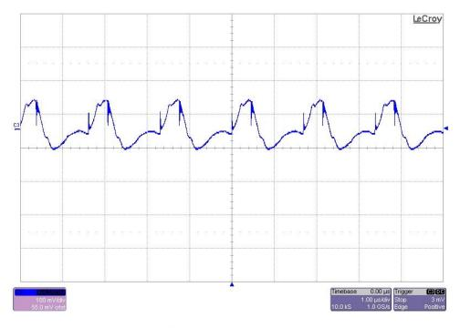
The output ripple voltage is shown in the figure below. The image was taken with the 15V output loaded to 1A and the input voltage set to 5.5V. (100mV/DIV, 1uS/DIV)
