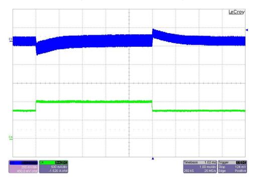
The photo below shows the 15V output voltage (ac coupled) when the load current is stepped between 0.5A and 1A. Vin = 5V. (200mV/DIV, 500mA/DIV, 1mS/DIV)
