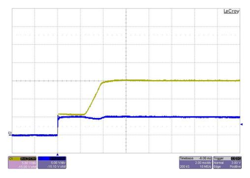
The photo below shows the output voltage startup waveform after the application of 5V in with the 15V output loaded to 1A. (5V/DIV, 2mS/DIV)
