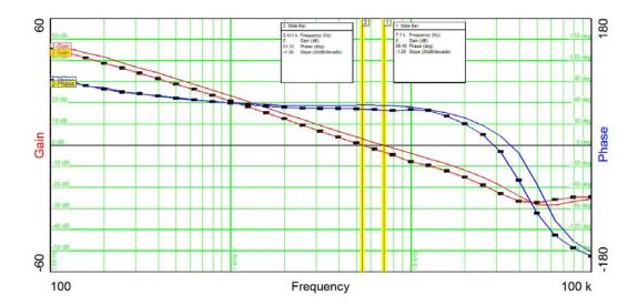
Loop response of the converter with a 300mA load:
