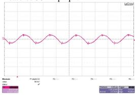
Input Ripple (C1), 12Vin 50mV/div, 1usec/div Measured 123mV pk-pk:
