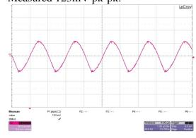
Output Ripple (C9), 24Vin 50mV/div, 1usec/div Measured 45mV pk-pk:
