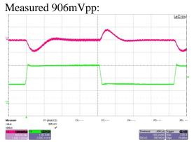
Load Step, 24Vin 1.5A to 3A step load 100mA/usec slew rate 200mV/div, 100usec/div
