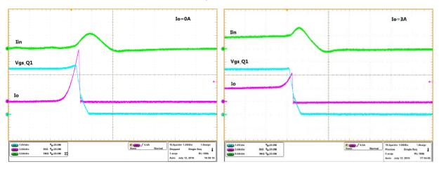
Figure 4. Output Short Circuit Performance at  $V_0=5V$  ( $V_{IN}=3.6V$ )
