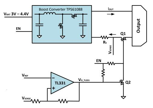
Figure 1. Block Diagram of PMP9779
