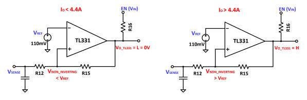
Figure 2. Comparator Circuit with Hysteresis
