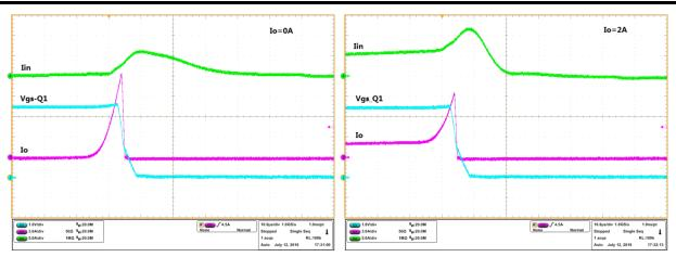
Figure 5. Output Short Circuit Performance at  $V_0=9V$  ( $V_{IN} = 3.6V$ )
