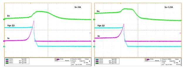
Figure 6. Output Short Circuit Performance at  $V_0=12V$  ( $V_{IN}=3.6V$ )
