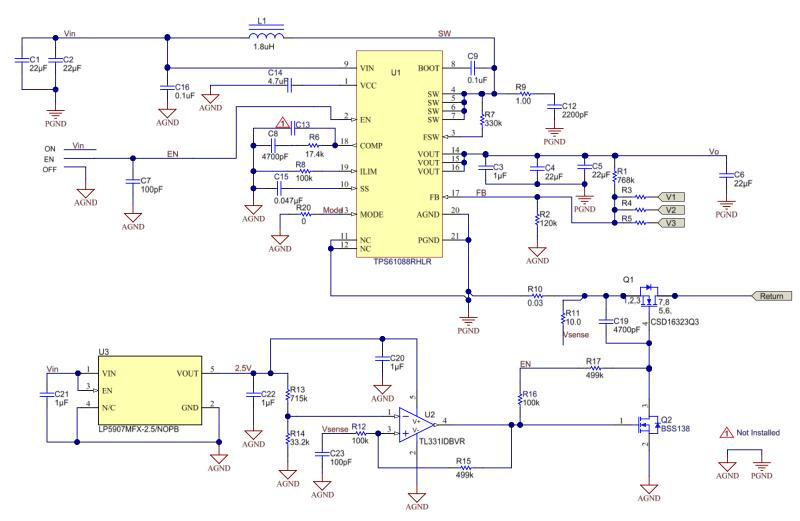
Figure 7. PMP9779 Schematic
