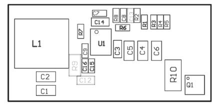
Figure 12. PMP9779 Top-side Assembly Drawing
