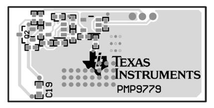
Figure 9. PMP9779 Bottom Layer and Bottom Silkscreen
