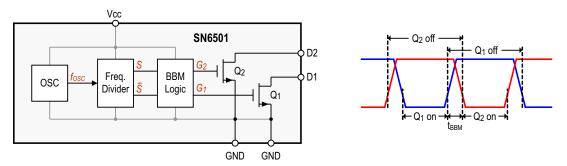
Figure 9. SN6501 Block Diagram
