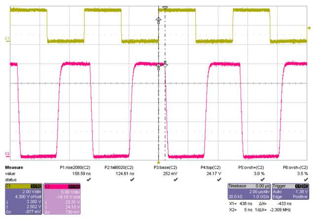
Figure 18. Output Waveform for 24-V Field Supply (No Cable)
