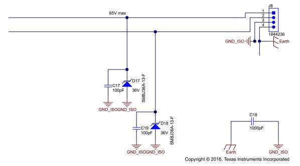
Figure 8. Protection TVS Diodes for Two Outputs
