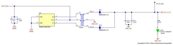
Figure 10. Push-Pull Circuit Schematic
