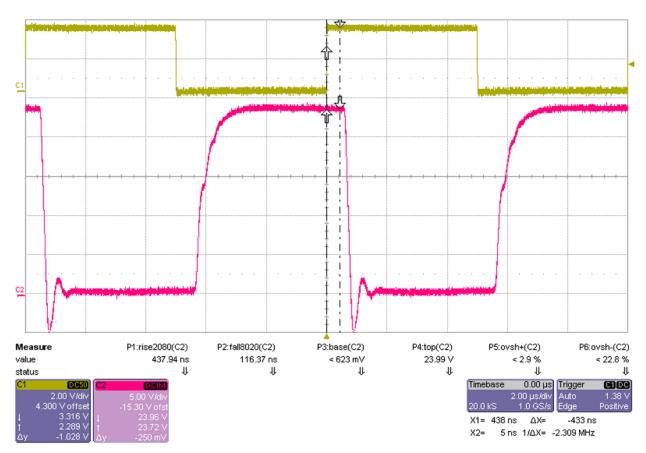
Figure 19. Output Waveform for 24 V Supply (With Cable)
