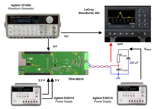
Figure 13. TIDA-00319 Test Setup
