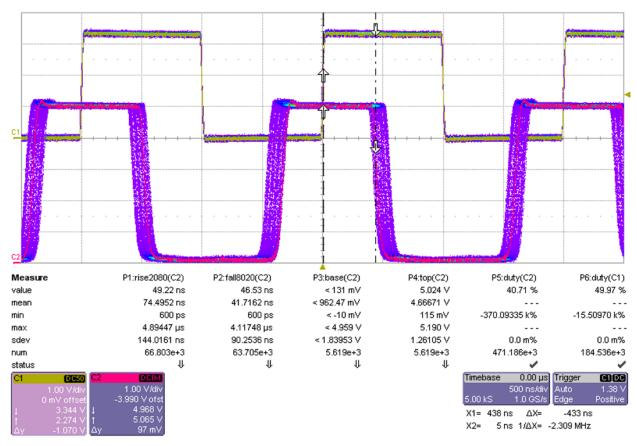
Figure 17. Delay Variation of Output Driver
