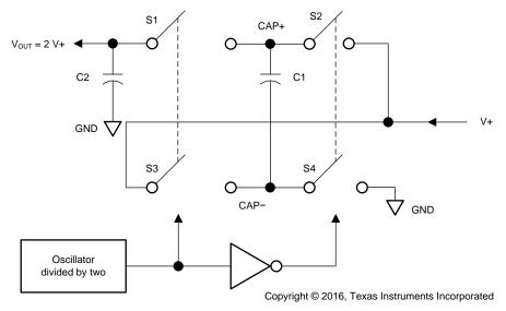
Figure 11. Voltage Doubling Principle
