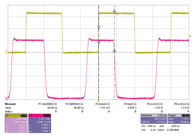
Figure 16. Output Waveform Without Cable at 500 kHz
