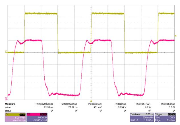
Figure 15. Output Waveform at 500 kHz With 15-m Cable
