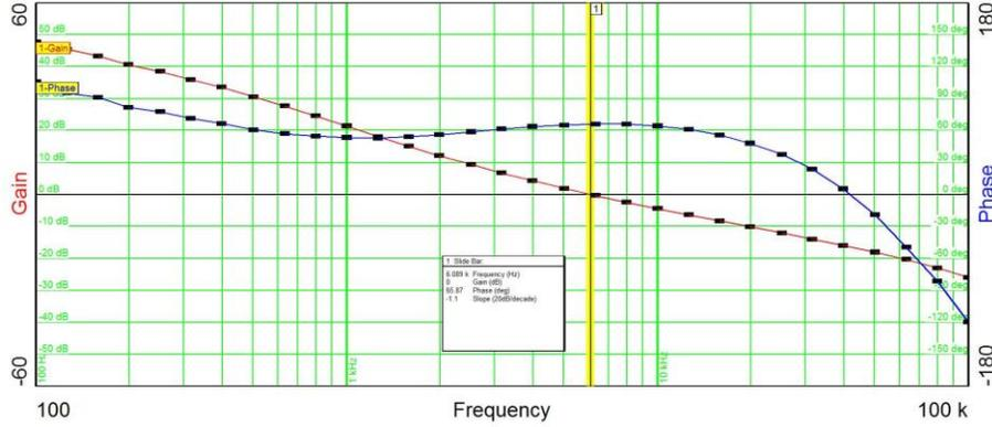
Loop response of the converter with a 48V input and 2A load
