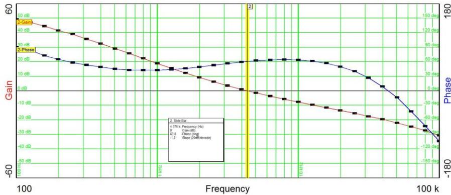
Loop response of the converter with a 48V input and 400mA load
