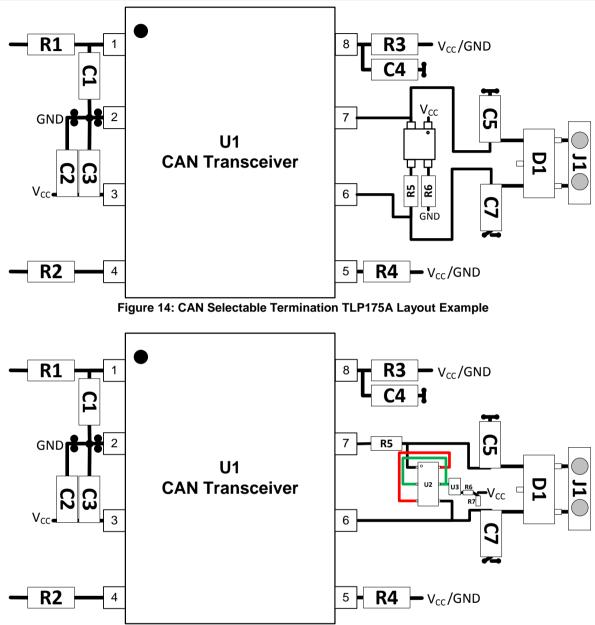
Figure 15: CAN Selectable Termination CSD87502Q2 and CSD17483F4 Layout Example
