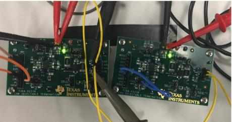
Figure 4: CAN Selectable Termination Evaluation Module FET Solution Setup
