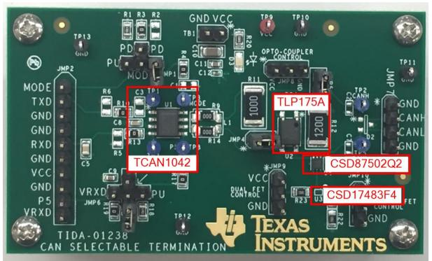
Figure 2: CAN Selectable Termination Evaluation Board Part Placement
