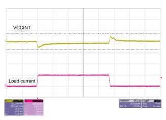
Figure 19. VCCINT Transient Response (5 V<sub>IN</sub>, 0- to 1-A Load Step)
