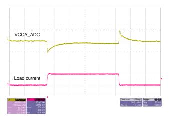
Figure 18. VCCA\_ADC Transient Response (5  $V_{IN}$ , 0- to 1-A Load Step)
