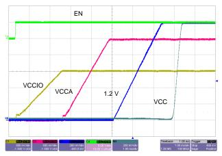
Figure 20. Startup on EN (5  $V_{\mbox{\tiny IN}},$  No Load, JP2 Open)
