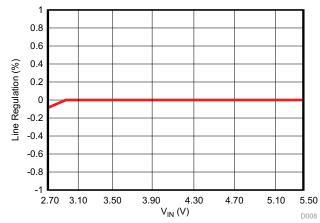
Figure 4. VCC Line Regulation (6-A Load, JP2 Shorted, Measured at J33)
