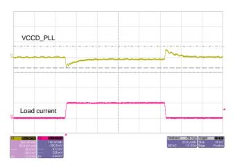
Figure 17. VCCD\_PLL Transient Response (5 V<sub>IN</sub>, 0- to 1-A Load Step)
