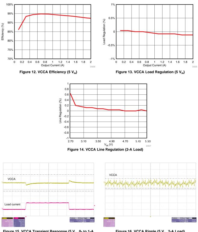
Figure 15. VCCA Transient Response (5 V<sub>IN</sub>, 0- to 1-A Load Step)
