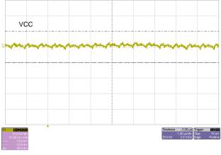
Figure 5. VCC Transient Response (5  $V_{IN}$ , 3- to 6-A Load Step, JP2 Shorted, Measured at J33)
