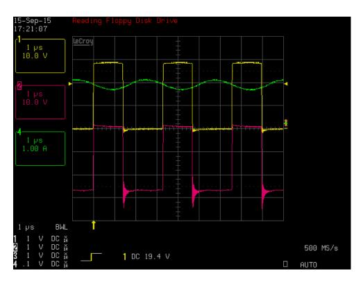
FET drain voltage and diode voltage and output current at 12 volts in
