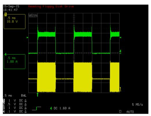
50% PWM dimming at 500 hz upper is (green) the LED current and the lower (yellow) is the FET drain. With 12 vdc input
