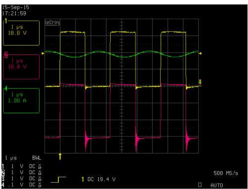
FET drain voltage and diode voltage and output current at 16 volts in
