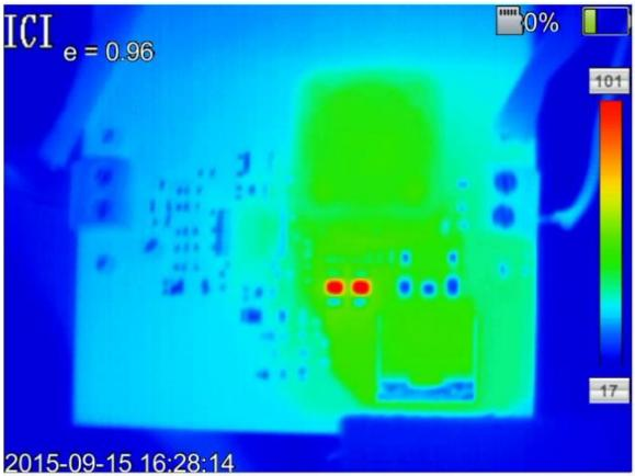
Worst case temperature is 100 deg C (current sense resistors) at full power
