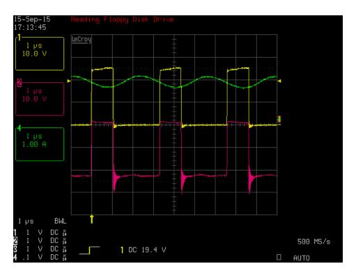
FET drain voltage and diode voltage and output current at 8 volts in
