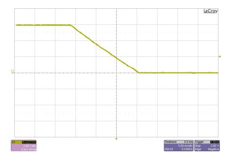
The photo below shows the turn off waveform of the 28V output, with a 100mA load, and an input voltage of 48V.
