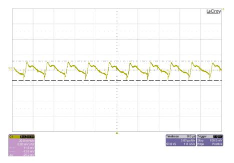
The picture below shows the output voltage ripple of the converter for the 28V output, with a full load of 2.5A. The input voltage is 48V.
