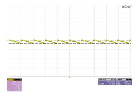
The picture below shows the output voltage ripple of the converter for the 28V output, with no load. The input voltage is 48V.
