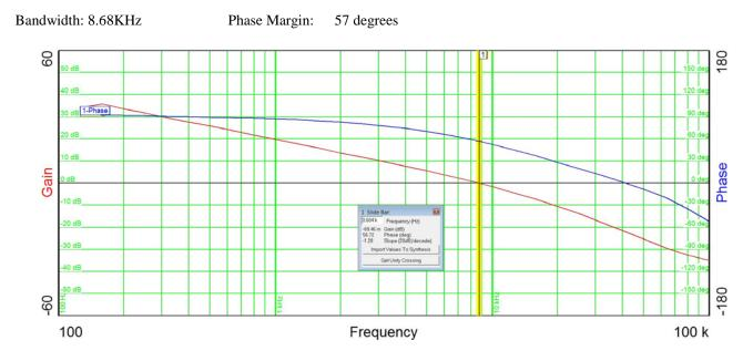
The frequency response below shows the 28V output with a full load of 2.5A.
