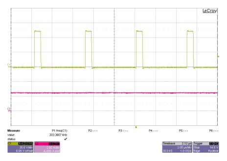
The picture below shows the switching waveform of the converter for the 28V output, with a full load of 2.5A. The input voltage is 48V and the frequency is shown to be 203 kHz.
