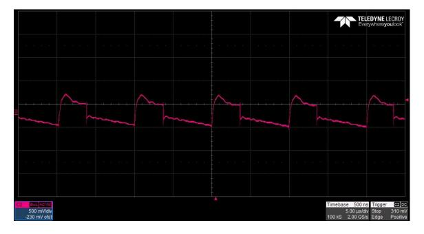
The 200V output ripple voltage (AC coupled) is shown in the figure below. The image was taken with the output loaded to 10mA. The input voltage is set to 15V. (500mV/DIV, 5uS/DIV)
