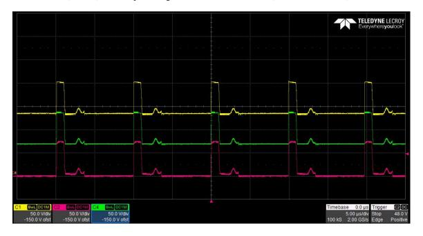
The photo below shows the FET switching voltage at TP4 (Red), the voltage at D2-cathode (Green) and D100-cathode (Yellow) for an input voltage of 15V and a 10mA load. (50V/DIV, 5uS/DIV)
