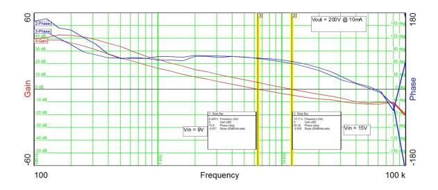
The plot below shows the loop gain with the input voltage set to 9V and 15V with the output set to 2mA.
