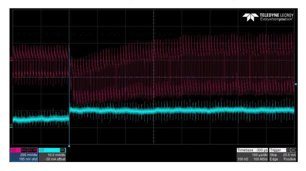
The photo below shows the 200V output voltage (ac coupled) when the load current is stepped between 10mA and 5mA. Vin = 12V. (200mV/DIV, 10mA/DIV, 100uS/DIV)
