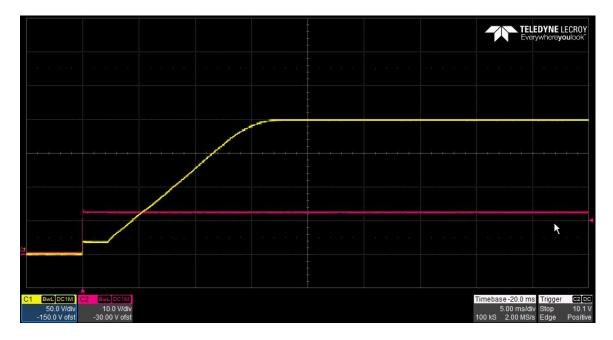
The photo below shows the output voltage startup waveform after the application of 12V in. The 200V output was loaded to 10mA. (Vin is 10V/DIV, Vout is 50V/DIV, 5mS/DIV)
