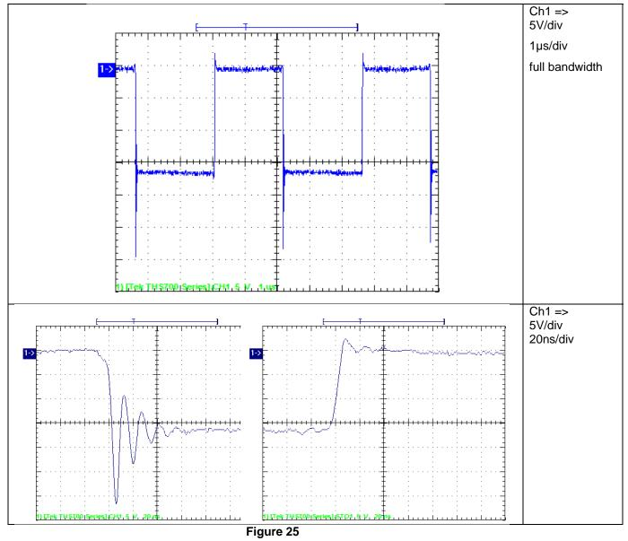
A 30V FET or a RC snubber is recommended for the synchronuous rectifier !
