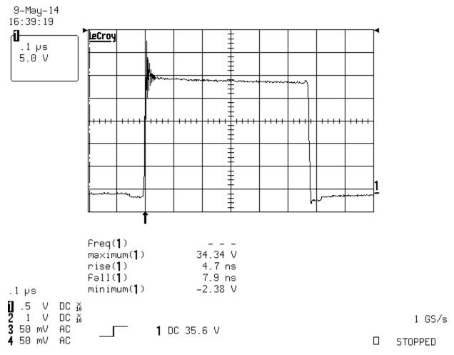
Figure 3. Switch Node, 4-A Load
