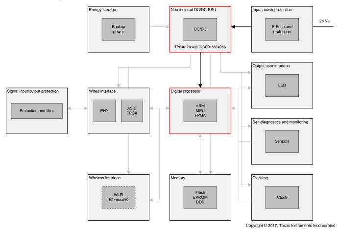
Figure 1. PMP15025 Block Diagram
