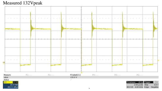
Drain voltage of Q1, 57V input and 3A load. 5V/div, 2.00uS/div, 750MHz bandwidth
