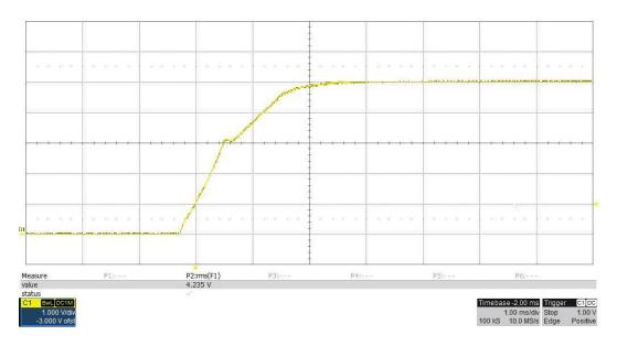
Output voltage startup waveform, 3A load 1V/ div, 1mS/ div
