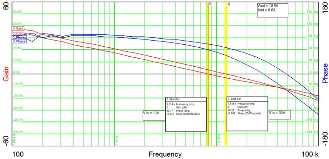
The plot below shows the 18.9V loop gain and phase margin with the output loaded to 0.1A.
