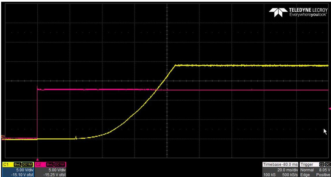
The photo below shows the 18.9V output voltage startup waveform (YELLOW) after the application of 30V in (RED) with the output loaded to 0A. (5V/DIV, 20mS/DIV)
