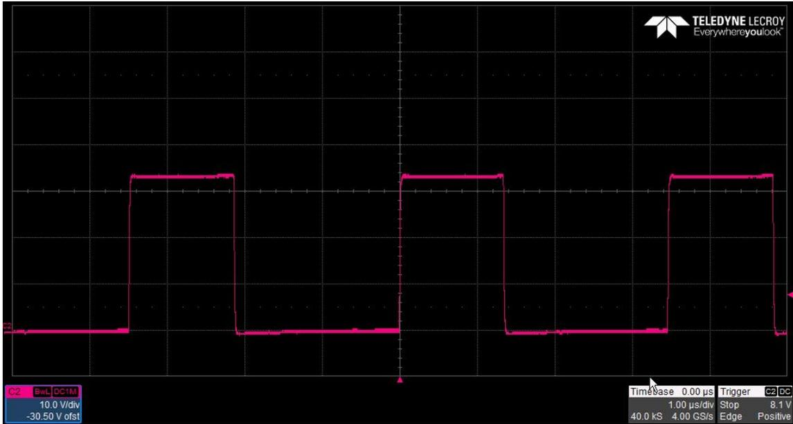
The photo below shows the SEPIC switch node voltage. The input voltage is 30V and the output is 18.9V @ 0.6A. (10V/DIV, 1uS/DIV)
