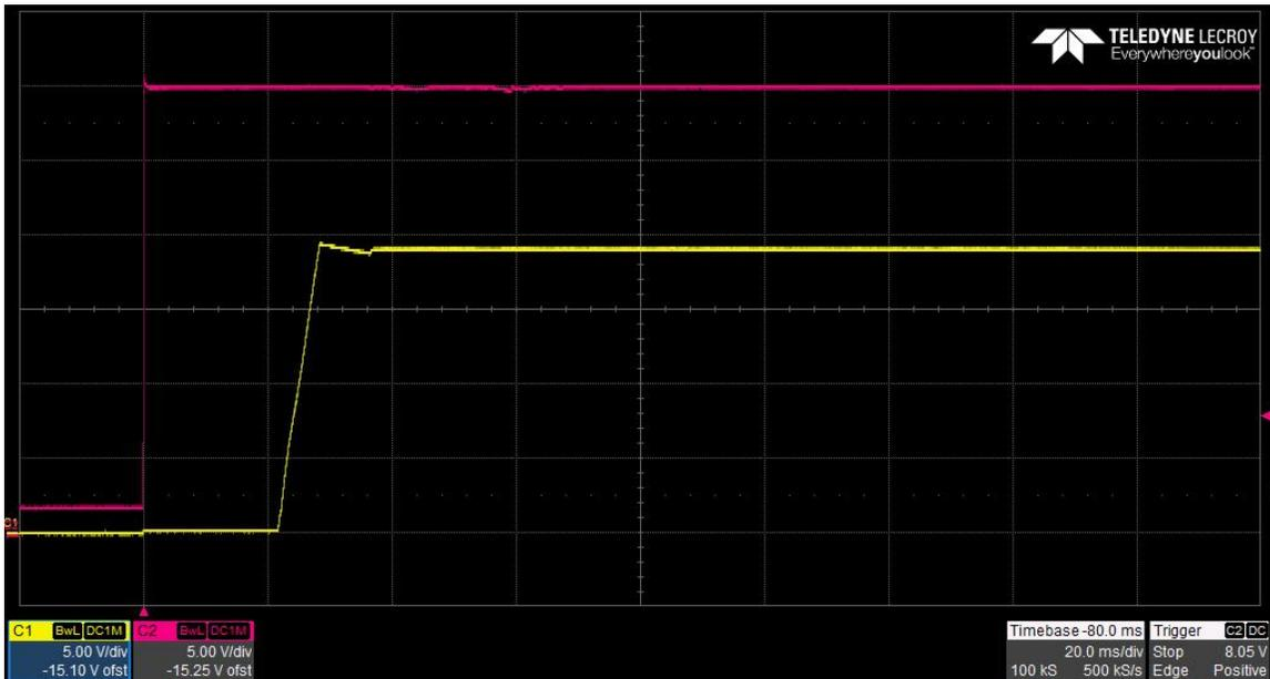
The photo below shows the 18.9V output voltage startup waveform (YELLOW) after the application of 30V in (RED) with the output loaded to 0.6A. (5V/DIV, 20mS/DIV)
