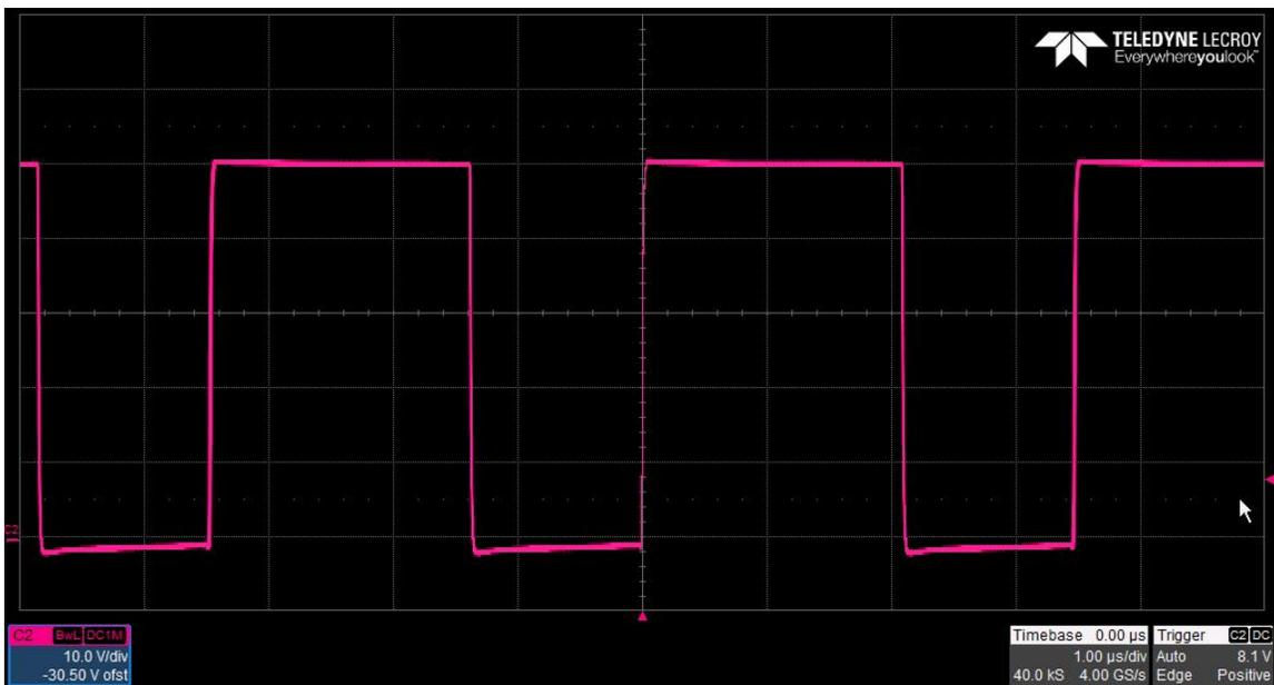
The photo below shows the SEPIC switch node voltage. The input voltage is 13V and the output is 18.9V @ 0.1A. The converter is operating in discontinuous mode. (10V/DIV, 1uS/DIV)
