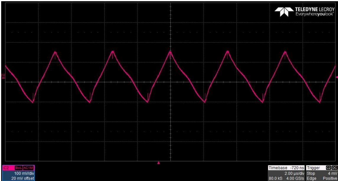
The 18.9V output ripple voltage (ac coupled) is shown in the figure below. The image was taken with the output loaded to 0.6A. The input voltage is set to 30V. (100mV/DIV, 2uS/DIV)
