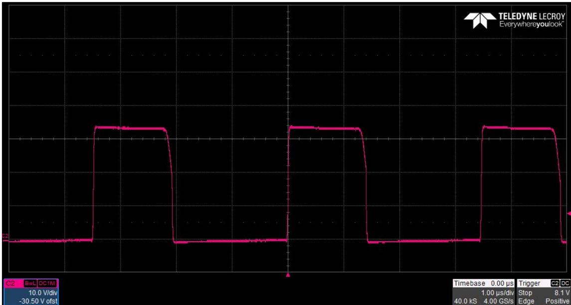
The photo below shows the SEPIC switch node voltage. The input voltage is 30V and the output is 18.9V @ 0.1A. The converter is operating in discontinuous mode. (10V/DIV, 1uS/DIV)
