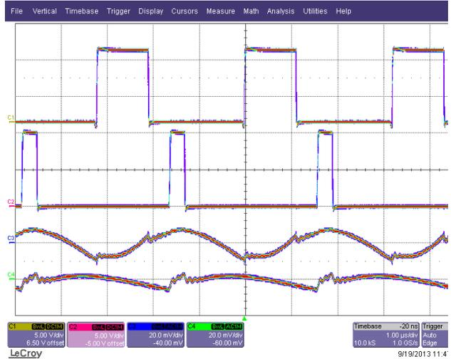
10VIN, Ch1 = 3.3V/8A, Ch2 = 1.0V/1A (2x 100uF, 6.3V, 1210+2x330uF, 6.3V, 9mohm, 7343), VOUT2=10mVpp
