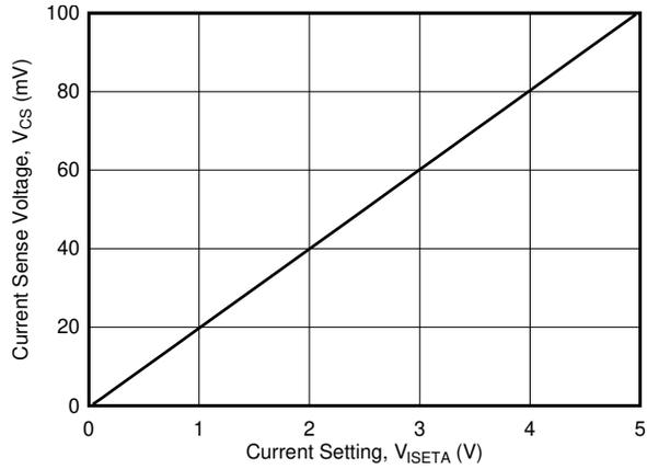
图 7-7. Regulated  $V_{CS}$  Voltage vs ISETA Voltage
