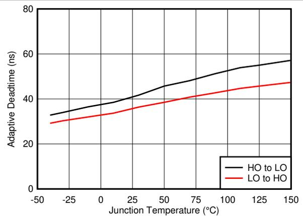
图 7-16. Adaptive Dead Time vs Temperature
