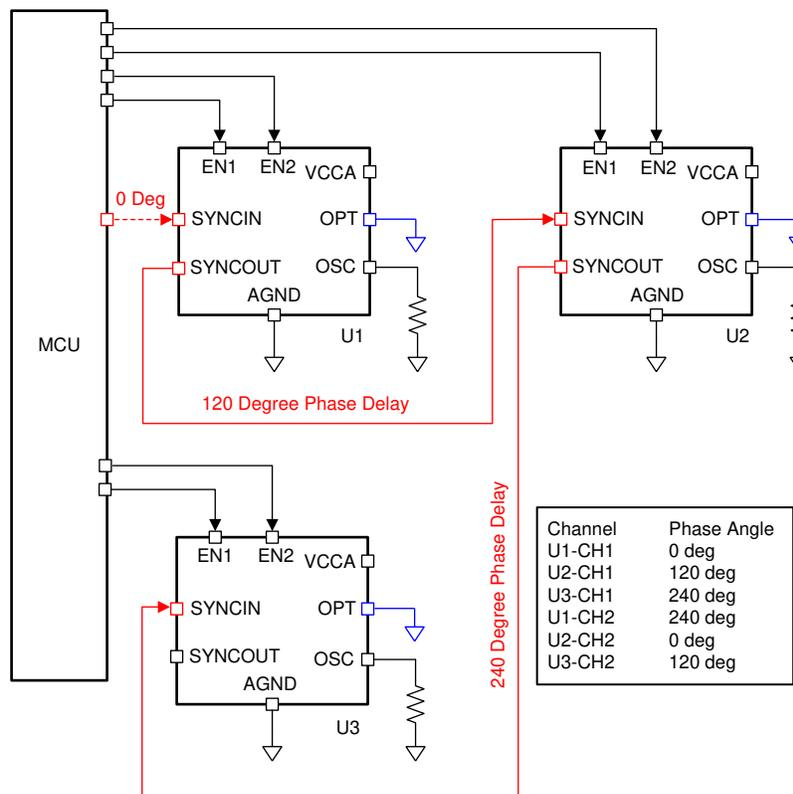
图 8-23. Six Phases 120° Interleaving Configuration
