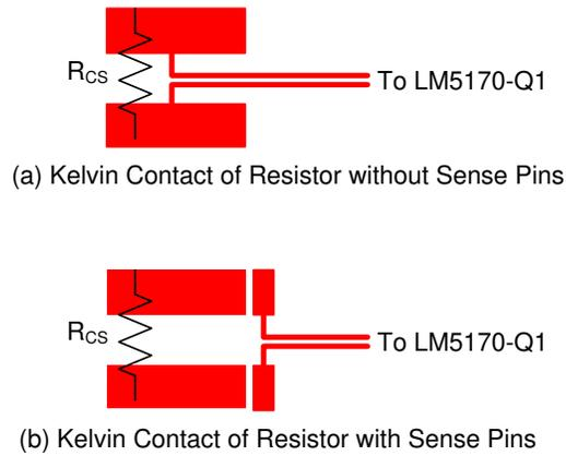
图 11-3. A Layout Example of Current Sense Routing
