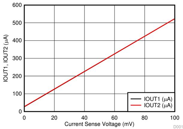
图 7-9. IOUT1/2 Current Monitor vs  $V_{CS}$  Voltage
