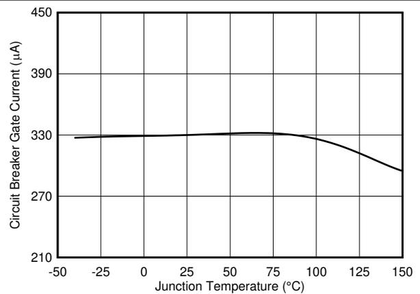
图 7-18. Circuit Breaker Gate Current vs Temperature
