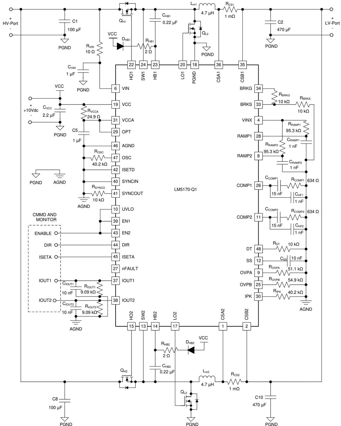
图 9-8. Schematic of the Example Dual-Phase Bidirectional Converter
