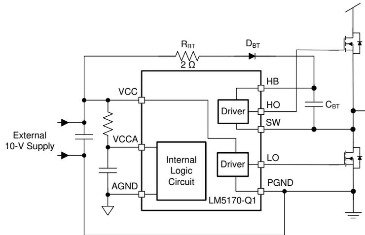
图 8-8. Bootstrap Circuit for High-Side Bias Supply
