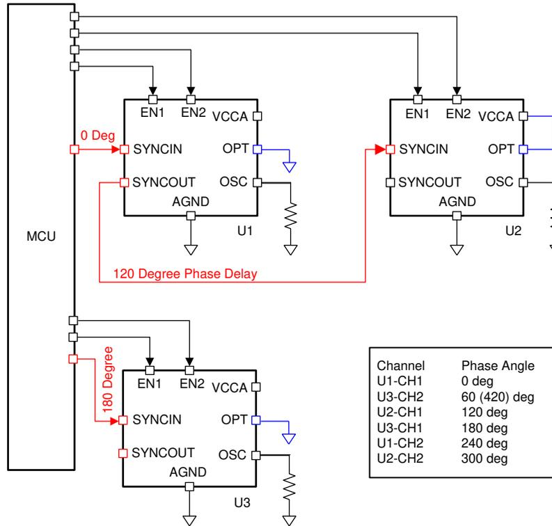
图 8-22. Six Phases 60° Interleaving Configuration
