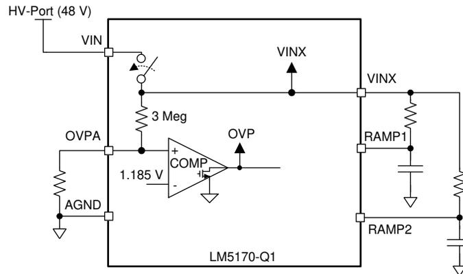
图 8-2. VIN and VINX Pins Configuration
