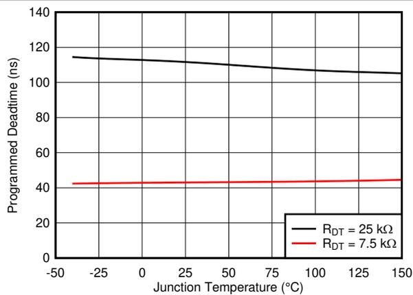
图 7-15. Programmed Dead-Time vs Temperature
