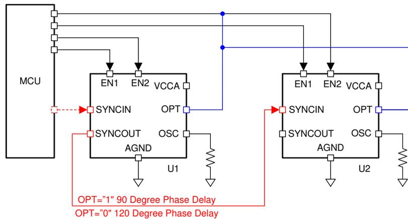
图 8-21. Three or Four Phases Interchangeable Configuration
