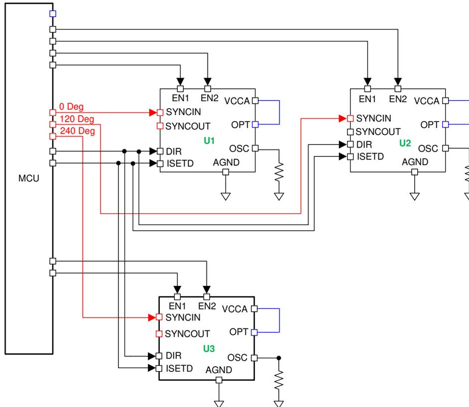
图 8-20. Example of Six Phase Star Configuration
