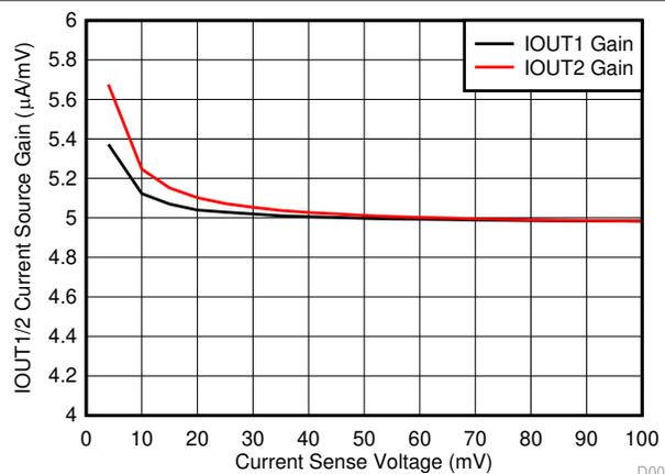
图 7-6. IOUT1/2 Current Monitor Accuracy vs  $V_{CS}$
