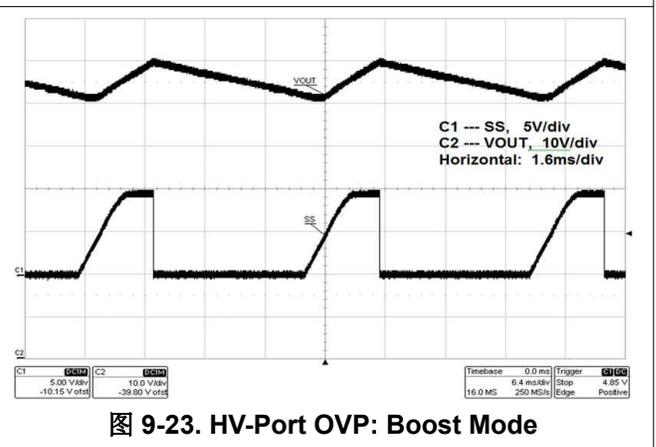
图 9-23. HV-Port OVP: Boost Mode
