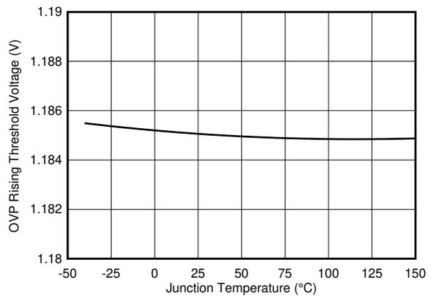
图 7-12. OVP Reference Voltage vs Temperature
