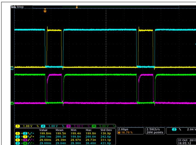
图 9-5. Bench Test Waveform for INA/B and OUTA/B
