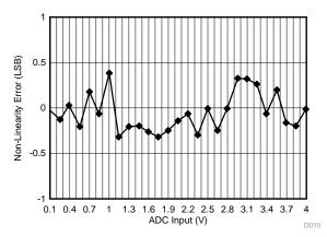
图 29. Measurement Data—ADC Linearity (26 Points)
