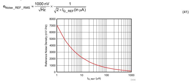
图 15. Characteristic Curve of Reference Noise versus Quiescent Current – Approximation of Noise Density for Band Gap References
