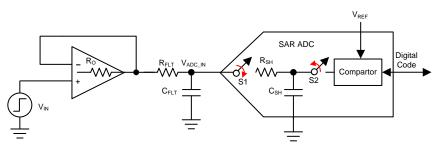
图 11. Simplified Schematic of Single-Ended ADC Input Stage
