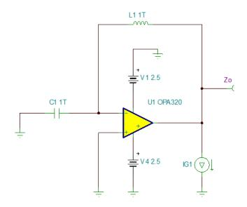
图 16. TINA-TI™ Schematic—Measuring Open-Loop Output Impedance of OPA320
