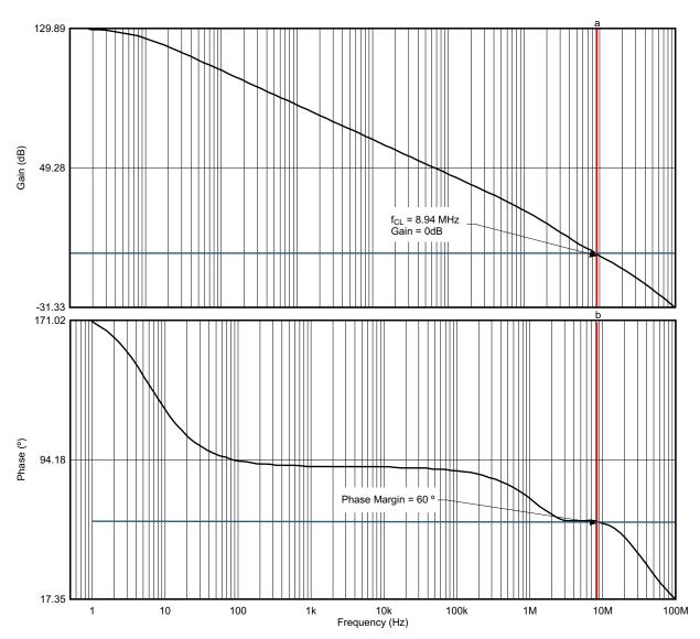
图 23. TINA-TI<sup>™</sup> Simulation Result—Loop Gain Magnitude and Phase Plot for Input Driver Stability
