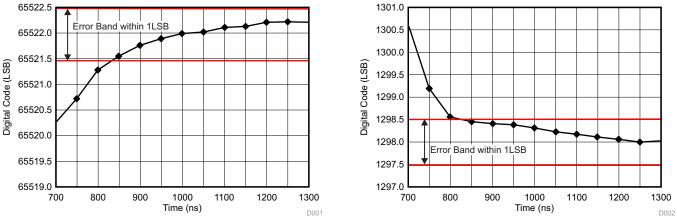
图 1. Measurement Result of Settling Time Plot for Multiplexed Data Acquisition Block<sup>(1)</sup> Rising Full-Scale Input and Falling Full-Scale Input
