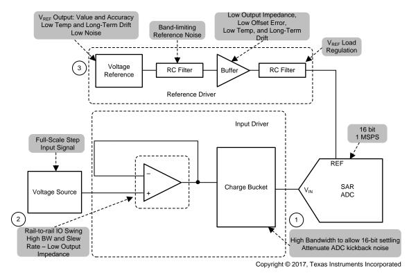
图 2. System Block Diagram Highlighting Primary Design Criteria
