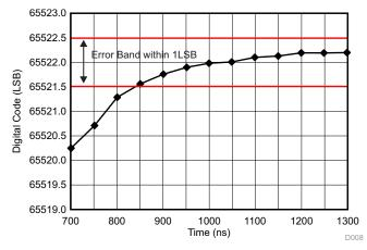
图 26. Measurement Data—Acquired Code in Different Settling Time for Rising Full-Scale Input
