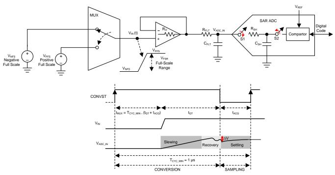
图 9. Timing Diagram of Settling Time in DAQ
