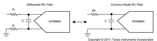
图 18. Design Configuration for Charge Bucket at ADC Input
