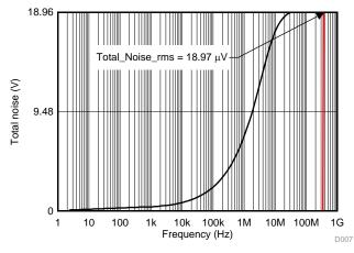
图 25. TINA-TI™ Simulation Result—Integrated Input Amplifier RMS Noise
