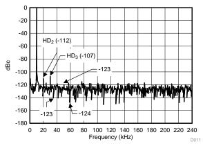
图 30. Measurement Data—FFT of DAQ Block
