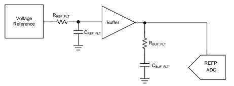
图 14. Block Diagram of Reference Driver
