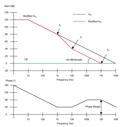
$\underline{\mathbb{8}}$  12. Analyzing Effect of RC-Filter on Op Amp Stability Using  $A_{oL}$  Response
