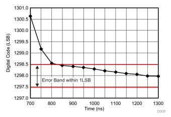
图 27. Measurement Data—Acquired Code in Different Settling Time for Falling Full-Scale Input
