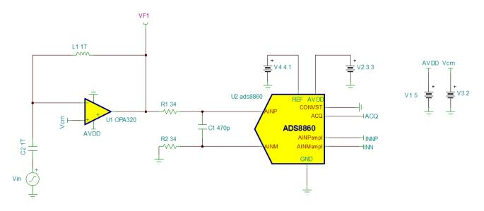
图 22. TINA-TI<sup>™</sup> Schematic—Checking Input Amplifier Stability
