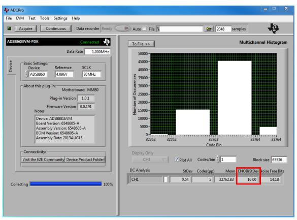
图 28. Measurement Data—Effective Resolution of DAQ Using ADCPro™
