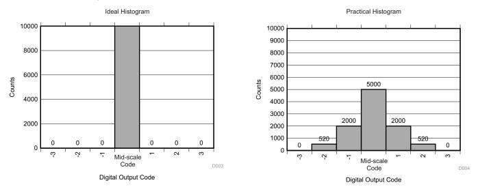
图 5. Histogram of ADC Output Codes for Constant Midscale DC Input
