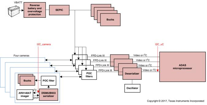
图 11. Setup for Monitoring I<sup>2</sup>C Transactions
