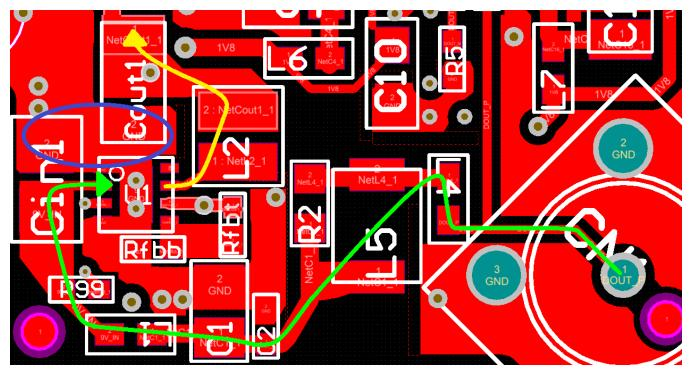
图 15. Routing FB Traces Around SW Nodes
