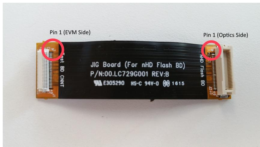
图 2. Overview of Flex Cable Pinout for 0.2 nHD Optical Engine
