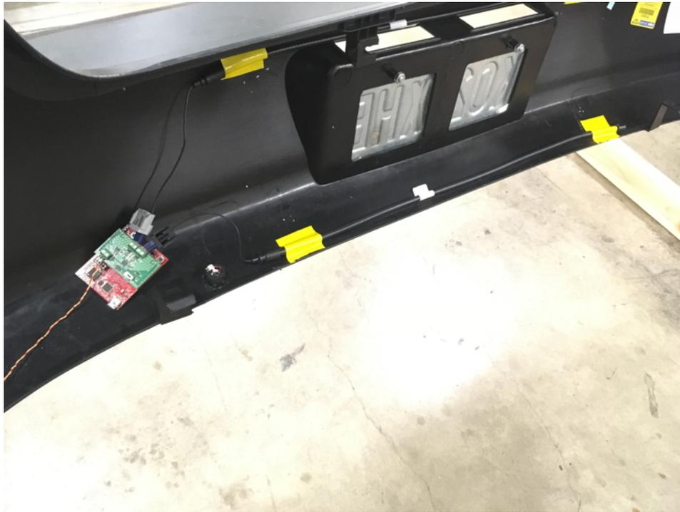
图 20. Capacitive Antennas Mounted on Bumper Cover
