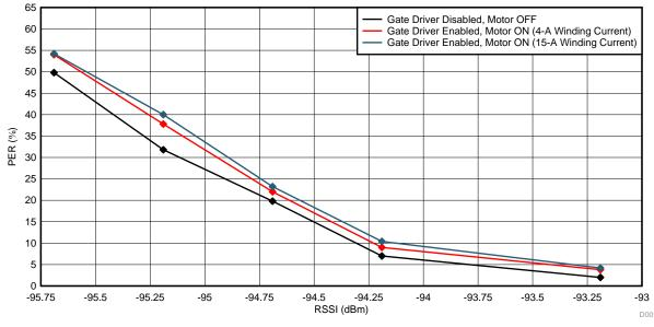
图 35. RX Sensitivity Measurement at 2402 MHz
