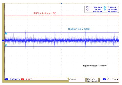
图 18. Output Voltage of 3.3 V From LDO and 3.3-V Voltage Ripple
