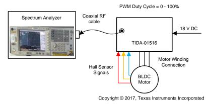
图 44. Test Setup to Evaluate TX Performance in Advertising Mode
