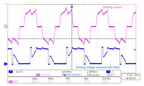
图 26. Motor Waveforms at 18-V DC Input, 27-A<sub>RMS</sub> Winding Current, 100% Duty Cycle
