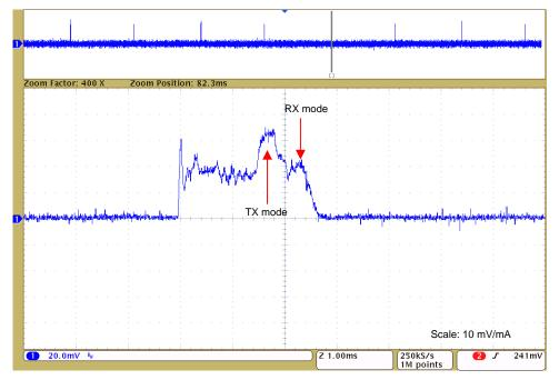
图 50. Bluetooth low energy Chip Current Consumption: 1-s Interval Connection Mode, BLE Only Mode
