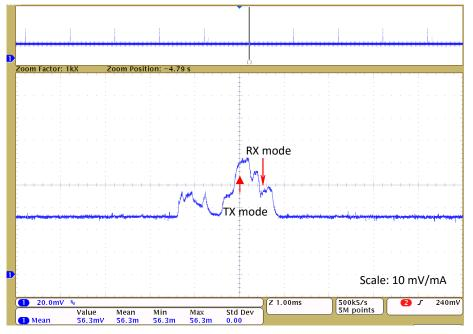
图 48. Bluetooth low energy Chip Current Consumption: 1-s Interval Connection Mode When Motor is Running
