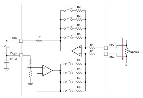
图 7. DRV8323 Current Shunt Amplifier Configuration
