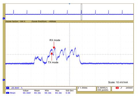
图 47. Bluetooth low energy Chip Current Consumption: Three-Channel 100-ms Interval Advertising Mode When Motor is Running
