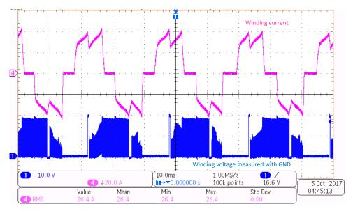
图 25. Motor Waveforms at 18-V DC Input, 26.4-A<sub>RMS</sub> Winding Current, 50% Duty Cycle
