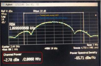
图 39. Measured TX Channel Power Measurement at 2440 MHz, 0-dBm Level With Motor ON and OFF
