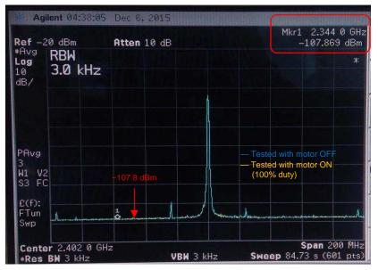
图 43. TX Performance With Bluetooth Channel Frequency of 2402 MHz
