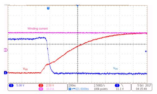
B 22. Turnon—High-Side  $V_{GS}$  and  $V_{DS}$  at 20-A Winding Current
