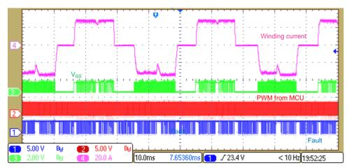
图 28. Cycle-by-Cycle Current Limit by DRV8323
