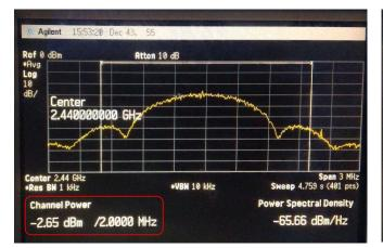
图 38. Measured TX Channel Power Measurement at 2440 MHz, 0-dBm Level
