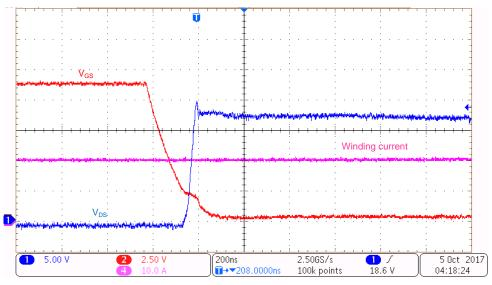
B 23. Turnoff—High-Side  $V_{GS}$  and  $V_{DS}$  at 20-A Winding Current
