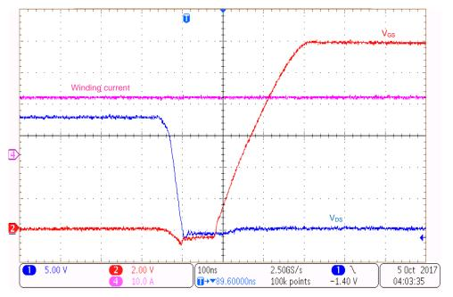
图 20. Turnon—Low-Side  $V_{GS}$  and  $V_{DS}$  at 20-A Winding Current
