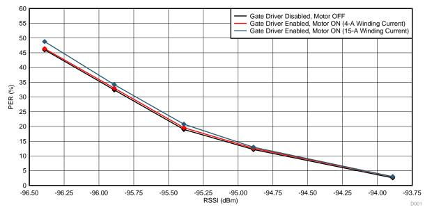
图 33. RX Sensitivity Measurement at 2480 MHz
