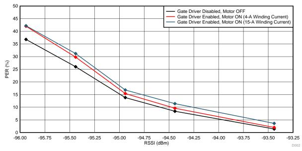
图 34. RX Sensitivity Measurement at 2440 MHz
