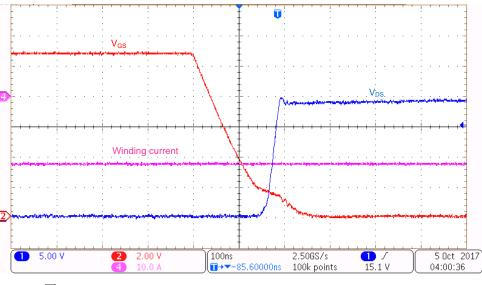
图 21. Turnoff—Low-Side V<sub>gs</sub> and V<sub>Ds</sub> at 20-A Winding Current
