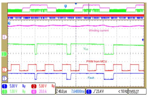
图 29. Cycle-by-Cycle Overcurrent Limit Showing PWM Shutoff
