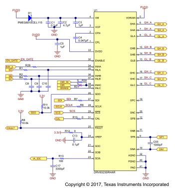
图 6. Schematic of DRV8323 Gate Driver
