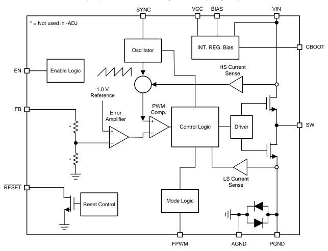
图 6. LMS3635-Q1 Functional Block Diagram
