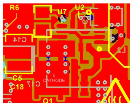
图 20. Reverse Battery Protection Layout
