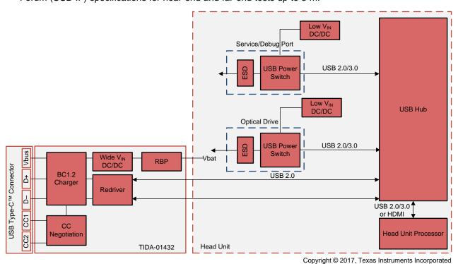
图 12. TIDA-01432 System Integration Concept
