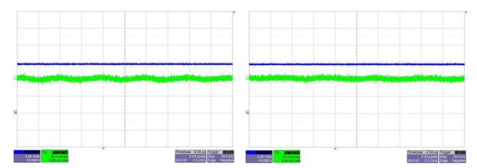
$\boxtimes$  37.  $V_{IN}$  = 14.5 V Measured at C13 With No Load
