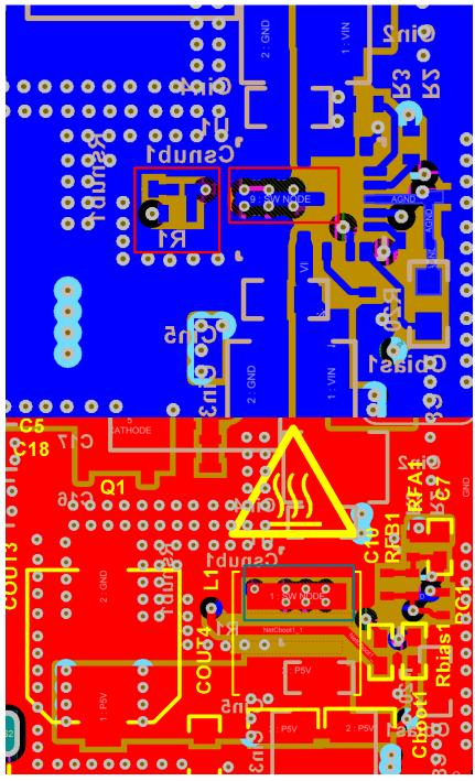
Note: The switch node is connected on the top and bottom of the board to minimize EMI and couple the thermals between the IC and inductor. A snubber and tuning resistor are also added.
