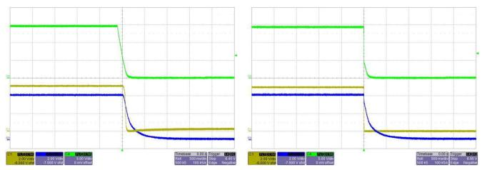
$\boxtimes$  28.  $V_{IN}$  = 14.5 V (Green), LMS3635 5  $V_{OUT}$  (Blue), USB 5 V (Yellow)—Shutdown = 150 ms at  $I_{OUT}$  = 0 A
