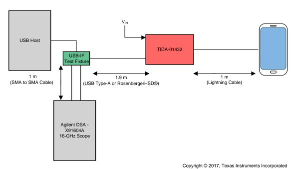
图 51. Block Diagram of Far-End Test Setup
