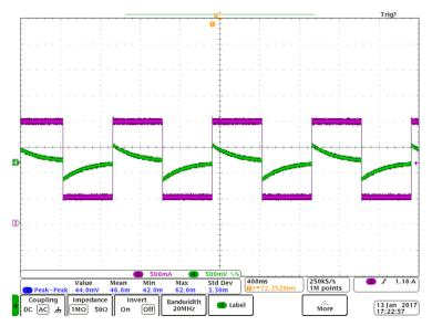
$\boxtimes$  33.  $V_{IN}$  = 13.5 V, Load Step = 0.5 A to 2 A (Switching), Load Transient = 250 mV at LMS3635  $V_{OUT}$  (COUT3)
