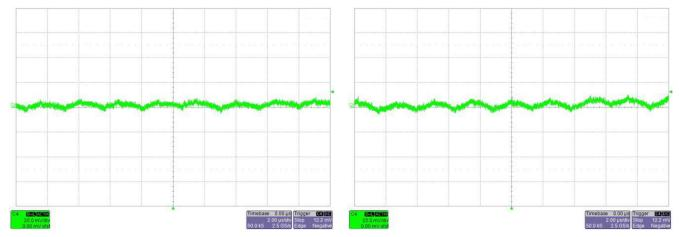
图 39. V<sub>IN</sub> = 14.5-V Output Ripple Measured at COUT3 With No Load
