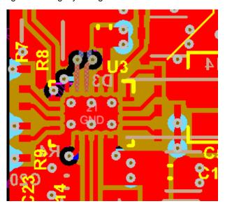
图 22. Legacy Charge Controller Layout
