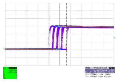
图 32. Spread Spectrum is ±3% of Switching Frequency
