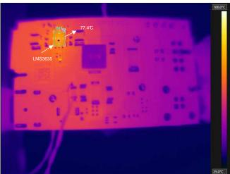
$\ \ \, \mbox{$\mathbb{R}$} \,$  44. LMS3635-Q1 IC at 77.4°C: V $_{\mbox{\tiny IN}} =$  14.5 V,  $\mbox{$\rm I_{\rm LOAD}$} =$  3 A, Soak Time = 20 min, Ambient Temperature 25°C
