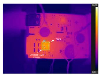
$\boxed{8}$  43. LMS3635-Q1 Output Inductor at 78.2°C:  $V_{IN}$  = 14.5 V,  $I_{LOAD}$  = 3 A, Soak Time = 20 min, Ambient Temperature 25°C
