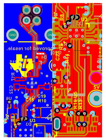
图 24. USB Redriver and Signal Routing Layout
