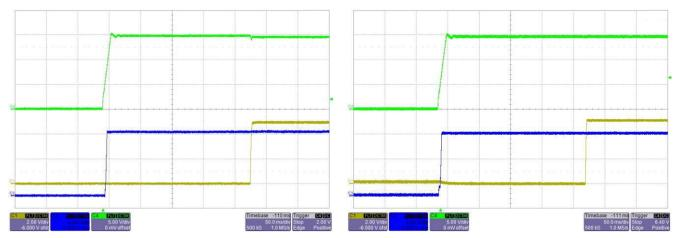
$\boxtimes$  26.  $\rm V_{IN}$  = 14.5 V (Green), LMS3635 5  $\rm V_{OUT}$  (Blue), USB 5 V (Yellow)—Start-Up = 15 ms at  $\rm I_{OUT}$  = 0 A
