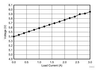
图 35. V<sub>IN</sub> = 14.5 Measured at C13, USB V<sub>OUT</sub> Measured at C16, Cable Compensation Enabled
