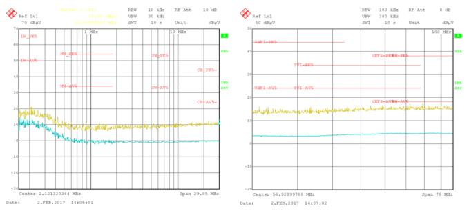
图 56. Low-Frequency Testing (100 kHz to 30 MHz) of Conducted EMI Performance
