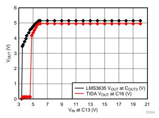
图 36.  $V_{IN}$  = 0 V to 20 V Measured at C13, 1.7- $\Omega$  Load
