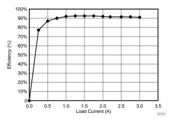
图 41. V<sub>IN</sub> = 14.5 V Measured at C13 With TIDA-01432 Efficiency—Measured at COUT3
