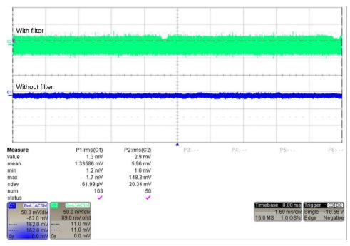
图 17. Output Noise During Silence Measurement
