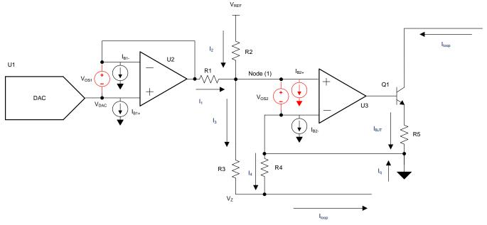
图 6. Transmitter V/I With Error Sources
