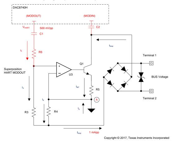
图 7. Superposition of HART Waveform
