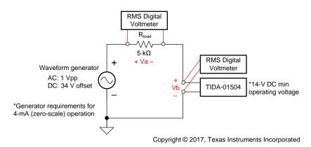
图 18. Test Setup of Transmitter Input Impedance
