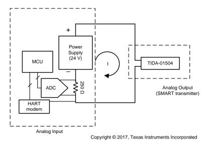
图 2. Example of Two-Wire Current Loop
