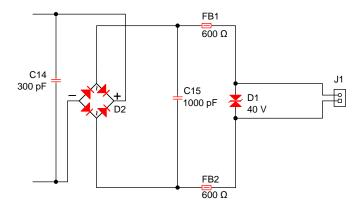
图 9. Diode Bridge Rectifier With TVS Protection Circuit
