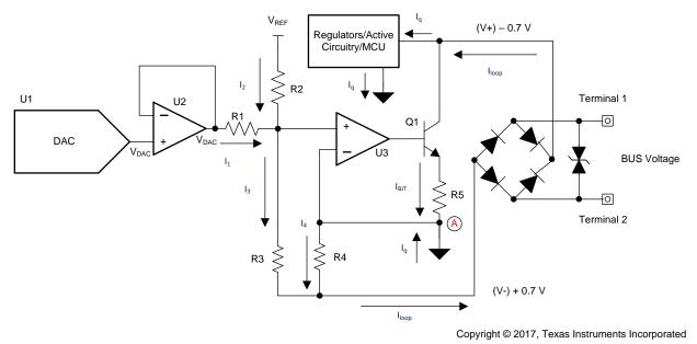
图 3. Simplified V/I Converter Circuit
