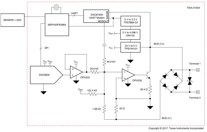
图 1. Detailed Circuit Diagram of TIDA-01504
