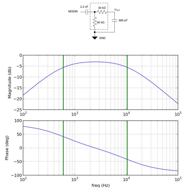
图 8. Band-Pass Filter and Frequency Response
