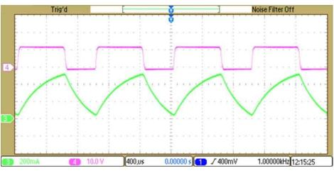
图 18. 60% Duty Cycle—Ch 4: Pulsating DC, Ch 3: Current Through Solenoid
