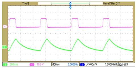
图 16. 20% Duty Cycle—Ch 4: Pulsating DC, Ch 3: Current Through Solenoid
