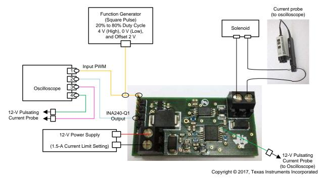
图 8. PWM Operation of Solenoid
