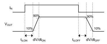
图 6. TPS1H100-Q1 Switching Characteristics Diagram
