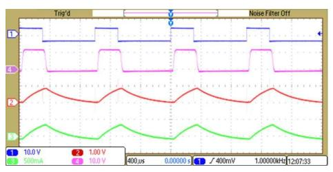
图 11. 30% Duty Cycle—Ch 1: Input PWM, Ch 2: INA240-Q1 Output, Ch 3: Current Probe Output, Ch 4: 12-V Pulsating
