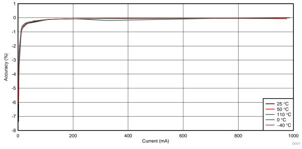
图 25. FS Accuracy at Different Temperatures
