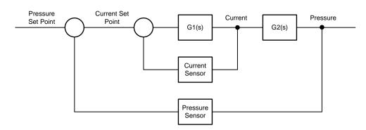
图 3. Closed-Loop Solenoid Control
