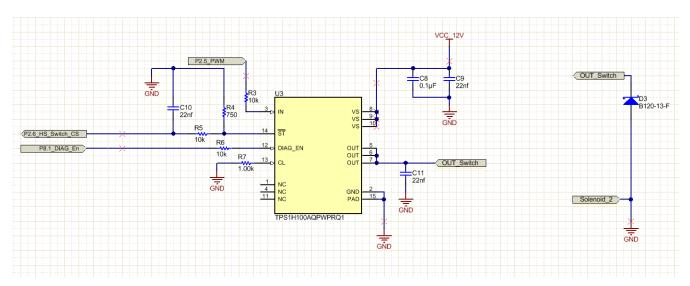
图 5. High-Side Switch Schematics
