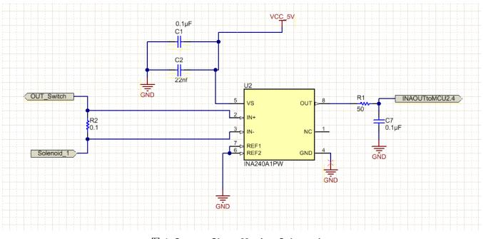
图 4. Current Shunt Monitor Schematics
