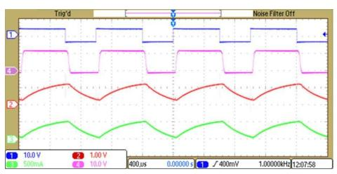
图 14. 60% Duty Cycle—Ch 1: Input PWM, Ch 2: INA240-Q1 Output, Ch 3: Current Probe Output, Ch 4: 12-V Pulsating
