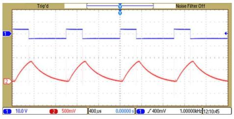
图 20. 40% Duty cycle—PWM Input versus Current Shunt Output, Ch 1: PWM Input, Ch 2: INA240-Q1 Output
