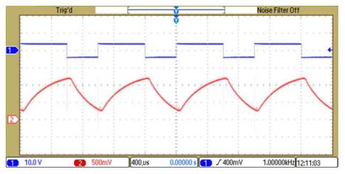
图 22. 60% Duty cycle—PWM Input versus Current Shunt Output, Ch 1: PWM Input, Ch 2: INA240-Q1 Output
