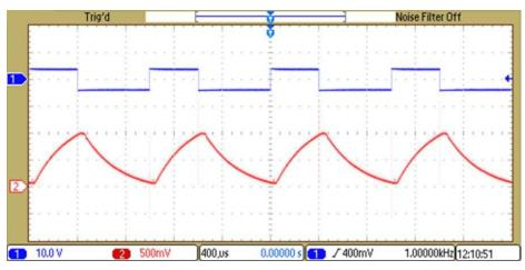
图 21. 50% Duty cycle—PWM Input versus Current Shunt Output, Ch 1: PWM Input, Ch 2: INA240-Q1 Output
