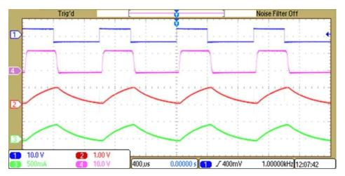
图 12. 40% Duty Cycle—Ch 1: Input PWM, Ch 2: INA240-Q1 Output, Ch 3: Current Probe Output, Ch 4: 12-V Pulsating
