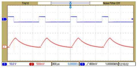
图 19. 20% Duty cycle—PWM Input versus Current Shunt Output, Ch 1: PWM Input, Ch 2: INA240-Q1 Output
