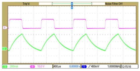
图 17. 40% Duty Cycle—Ch 4: Pulsating DC, Ch 3: Current Through Solenoid
