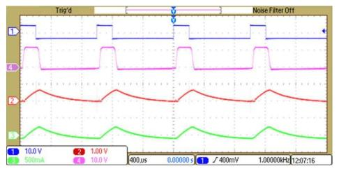
图 10. 20% Duty Cycle—Ch 1: Input PWM, Ch 2: INA240-Q1 Output, Ch 3: Current Probe Output, Ch 4: 12-V Pulsating
