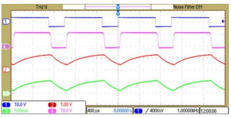
图 15. 70% Duty Cycle—Ch 1: Input PWM, Ch 2: INA240-Q1 Output, Ch 3: Current Probe Output, Ch 4: 12-V Pulsating
