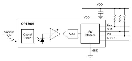
图 7. OPT3001 Functional Block Diagram
