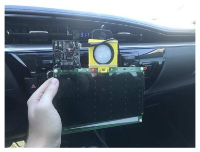
图 32. TIDA-01008 Outdoor Brightness—Center Stack Display in Vehicle
