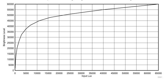
图 27. TIDA-01008 Ambient Lux to Backlight Brightness
