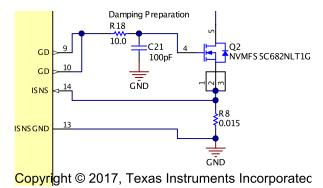
图 17. TIDA-01008 Schematic: Gate Resistor and Capacitor
