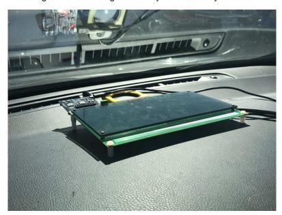
图 33. TIDA-01008 Outdoor Brightness—Front Dash of Vehicle
