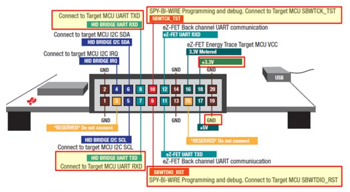
图 25. Programmer Connector Pinout
