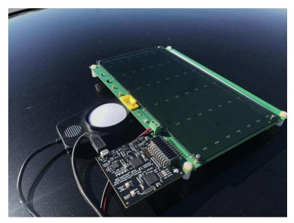
图 34. TIDA-01008 Outdoor Brightness—Outdoors (Top of Vehicle)
