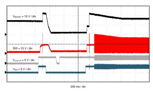
图 39. TIDA-01008 Start-Up Sequence With Residual Voltage
