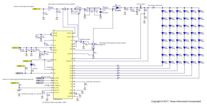
图 15. TIDA-01008 Schematic Backlight, Boost, and LED
