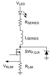
图 7. Parasitic Inductance ( $L_{series}$ ) and Resistance ( $R_{series}$ ) in Series With LED
