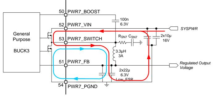
图 5. High AC Current Paths in a Buck Converter
