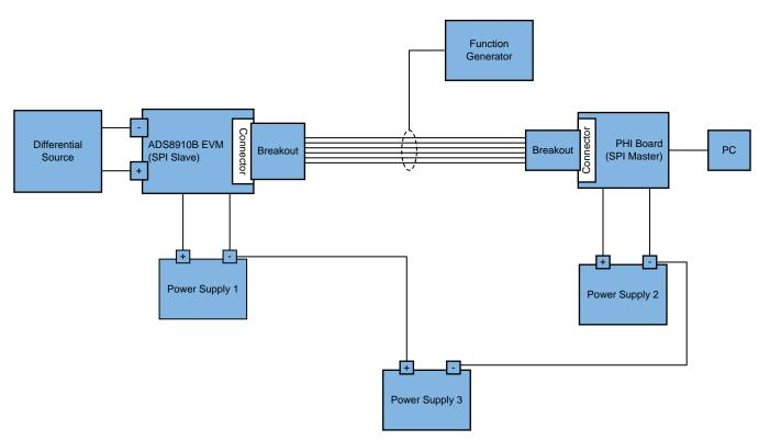
图 12. Single-ended SPI Test Setup
