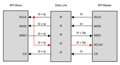
图 8. Feed SCLK back to SPI Master
