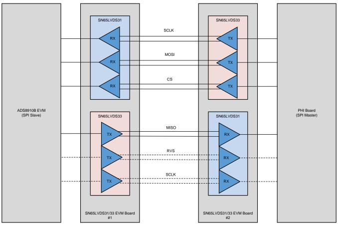
图 7. Eliminating Round-Trip Delay Block Diagram
