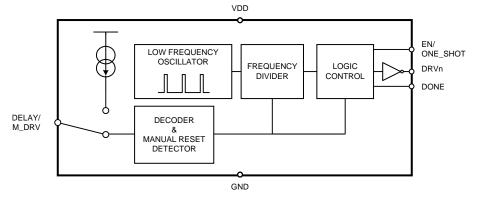
图 5. TPL5111 Functional Block Diagram
