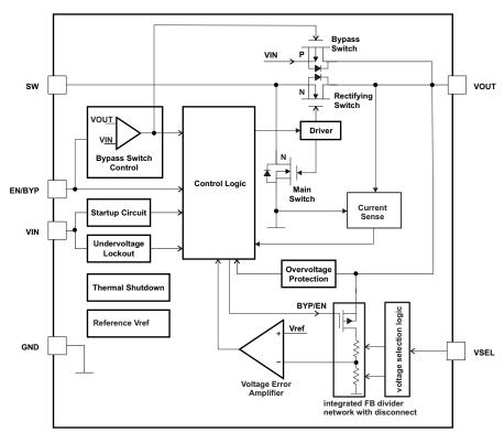
图 6. TPS61291 Functional Block Diagram
