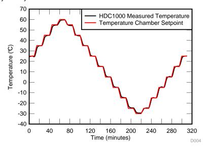
图 20. HDC1000 Measured Temperature Data and Environmental Chamber Set-Point
