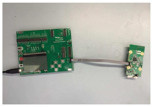
图 10. Connection of SmartRF06 Evaluation Board and TI Designs Hardware for Programming and Debugging
