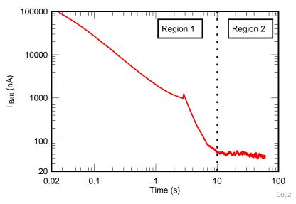
图 15. Off-State Current Versus Time
