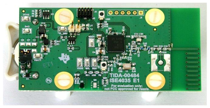
图 9. Humidity and Temperature Sensor Node for Sub-1GHz Star Networks Enabling 10+ Year Coin Cell Battery Life Reference Design Hardware
