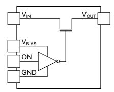
图 7. TPS22860 Functional Block Diagram
