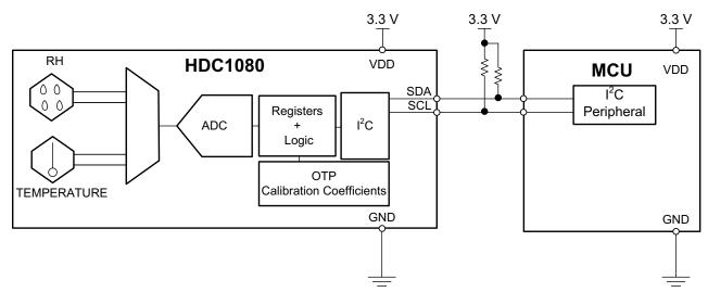
图 3. HDC1080 Functional Block Diagram
