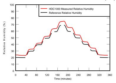
图 18. HDC1000 Measured Relative Humidity Data
