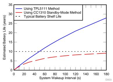
图 16. Estimated Battery Life Comparison: TPL5111 Nano-Power System Timer Versus CC1310 Standby Mode
