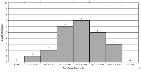
图 12. Zero-Scale Error Measurement
