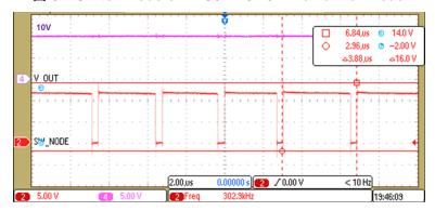
₹ 38 through ₹ 40 show the switch node performance of the boost converter, TPS61170, generating 8 V, 10 V, and 24 V for encoder supply.
