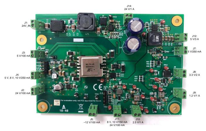
The TIDA-010009 is a compact board with 114-mm  $\times$  77.47-mm dimensions. 表 2 provides details on the connectors used in the design.
