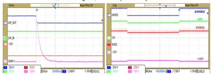
图 59. Shorting 24-V, 100-mA Output Rail of Flyback
