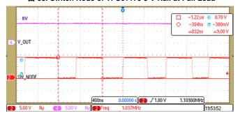
图 39. Switch Node of TPS61170 10-V Rail at Full Load
