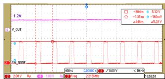
The following figures show the switch node performance of the buck converter, TPS62125, generating 5 V, 8 V, and 10 V for encoder supply.
