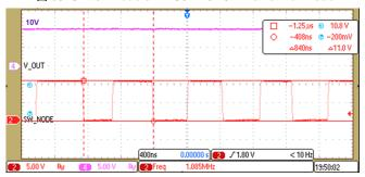
图 40. Switch Node of TPS61170 24-V Rail at Full Load
