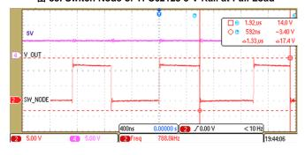
图 36. Switch Node of TPS62125 8-V Rail at Full Load
