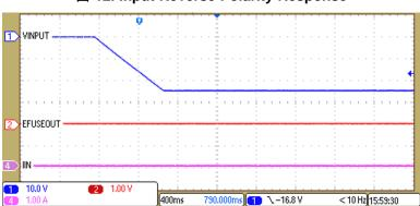
图 12. Input Reverse Polarity Response
