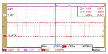
图 33. Switch Node of TPS62821 2.5-V Rail at Full Load
