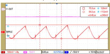
图 58. Output Ripple on -12-V Rail
