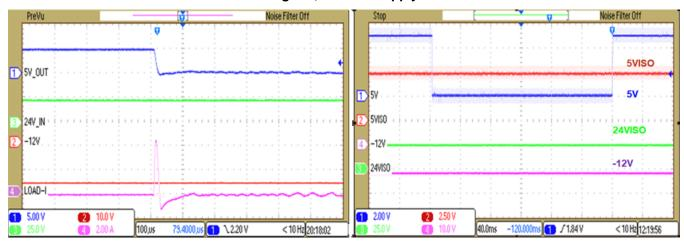
图 61. Shorting 8-V, 250-mA Supply to Encoder
