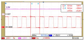
图 34. Switch Node of TPS62821 1.2-V Rail at Full Load
