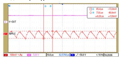
图 57. Output Ripple on Isolated 5-V Rail at Full Load
