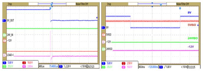
图 62. Shorting 10-V, 250-mA Supply to Encoder
