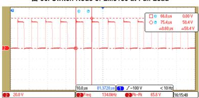
图 56. Switch Node of LM5180 at Full Load
