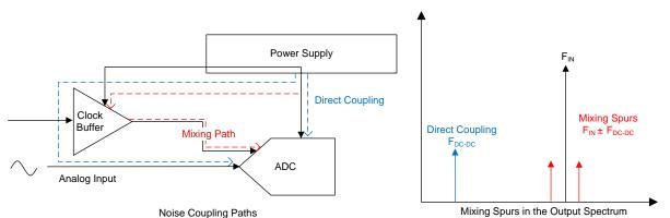
2. Impact of noise in clock generators: Noise floor and phase noise at the output of the clock generator is mainly affected due to two reasons:
