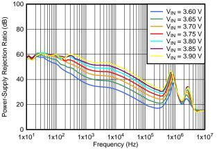
IOUT = 3 A, COUT = 47  $\mu\text{F}$  || 10  $\mu\text{F}$  || 10  $\mu\text{F}$ , CNR/SS = 10 nF, CFF = 10 nF
