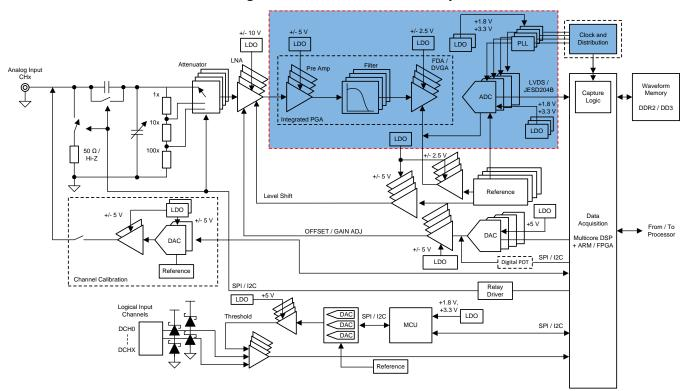
图 1. High-Performance DSO AFE Subsystem
