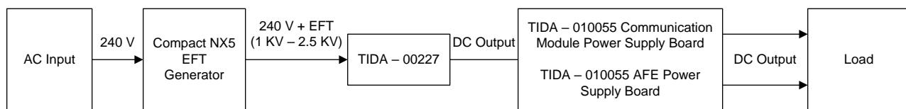
图 19 shows the TIDA-010055 power supply board for communication module interfaced to the TIDA-00227 reference design.
