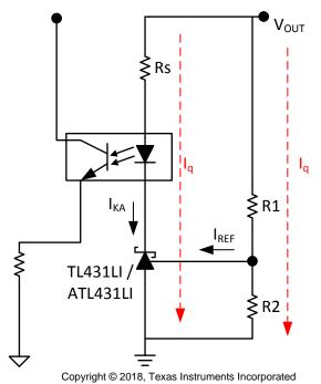
Figure 2. Current Paths in the Secondary Control Loop
