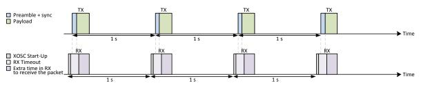
Figure 28: eWOR Mode (RX and TX in sync.)
