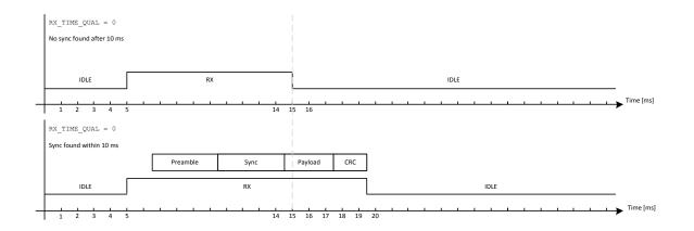
Figure 24: RX Termination when RX\_TIME\_QUAL = 0 (RX Timeout = 10 ms)
