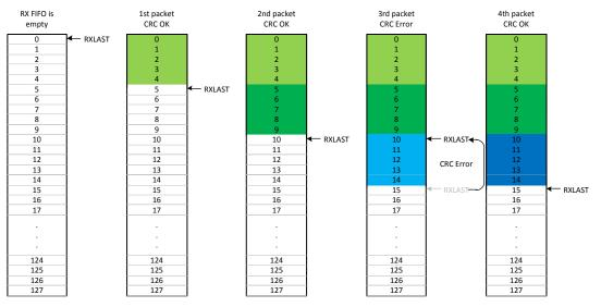
Figure 22: CRC Autoflush of Faulty Packet
