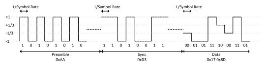
Figure 9: Data Sent Over the Air (CFM\_DATA\_CFG.SYMBOL\_MAP\_CFG = 0)
