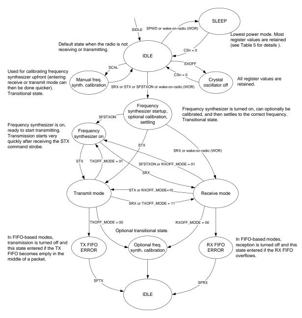
Figure 2: Simplified State Diagram
