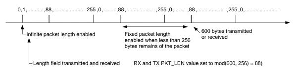
Internal byte counter in packet handler counts from 0 to 255 and then starts from 0 again
