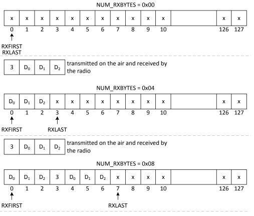
Figure 7: FIFO Pointers (RX FIFO) (1)
