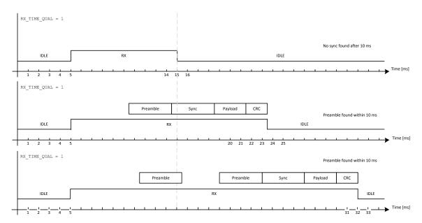
Figure 25: RX Termination when RX TIME QUAL = 1 (RX Timeout = 10 ms)
