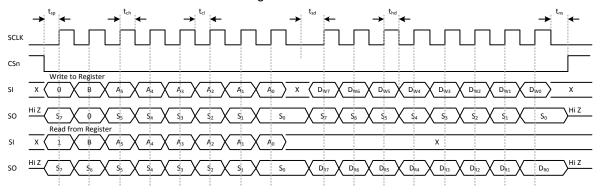
Figure 3: Configuration Registers Write and Read Operations
