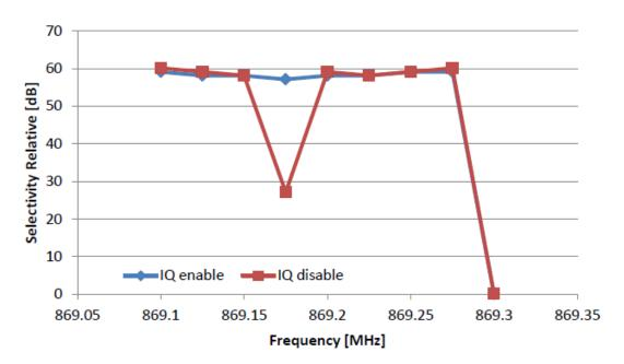
Figure 14: IQIC Enabled/Disabled (image at -125 kHz offset)
