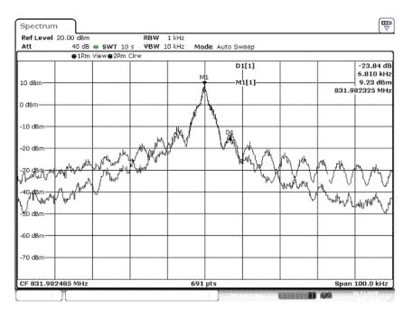
Figure 10: OOK with and without Shaping
