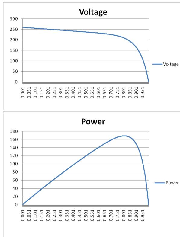
Figure 1. Example Panel Emulator Characteristics
