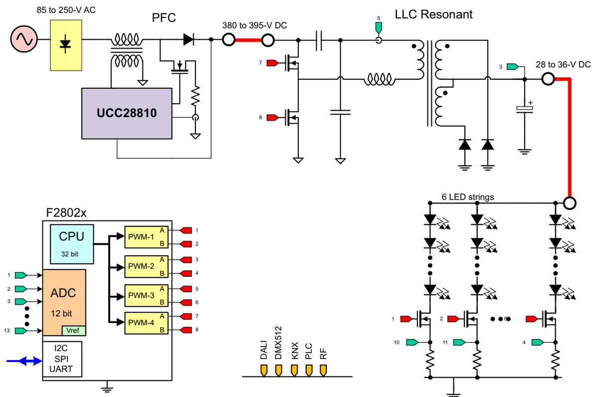
Figure 2. Block Diagram
