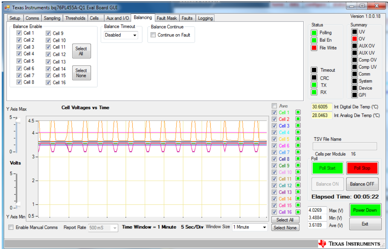
Figure 18. Cell Voltage Waveform When Cell 14 is Being Charged With 3.5 A
