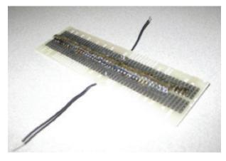
**Figure 2.** Our first unshielded 4000 µF AC-coupling capacitor for making noise measurements.
