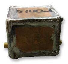
Figure 3. Our shielded 5100 uF AC-coupling cap which is used for making low noise measurements.
