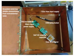
Figure 4. Test setup in shielded box.
