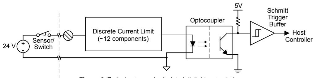
**Figure 6.** Typical optocoupler-isolated digital input solution.
