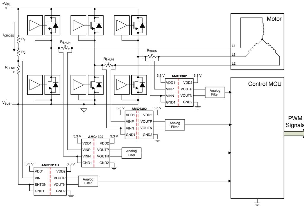
**Figure 5.** Typical current and voltage feedback implementation.
