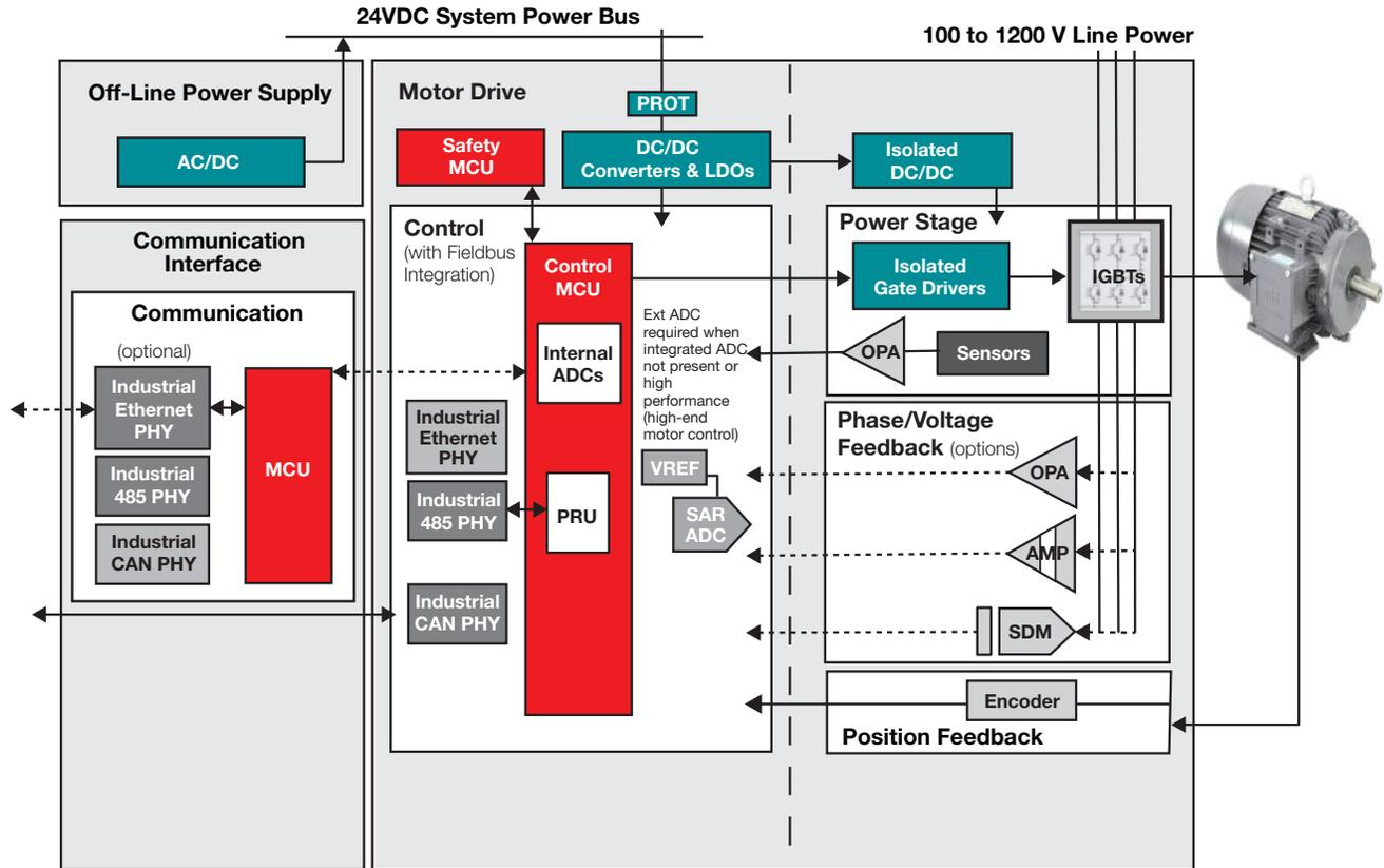
Figure 2. Block diagram of an AC motor drive.
