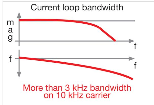
*Figure 2. Improving current loop bandwidth while maintain carrier frequency.*
