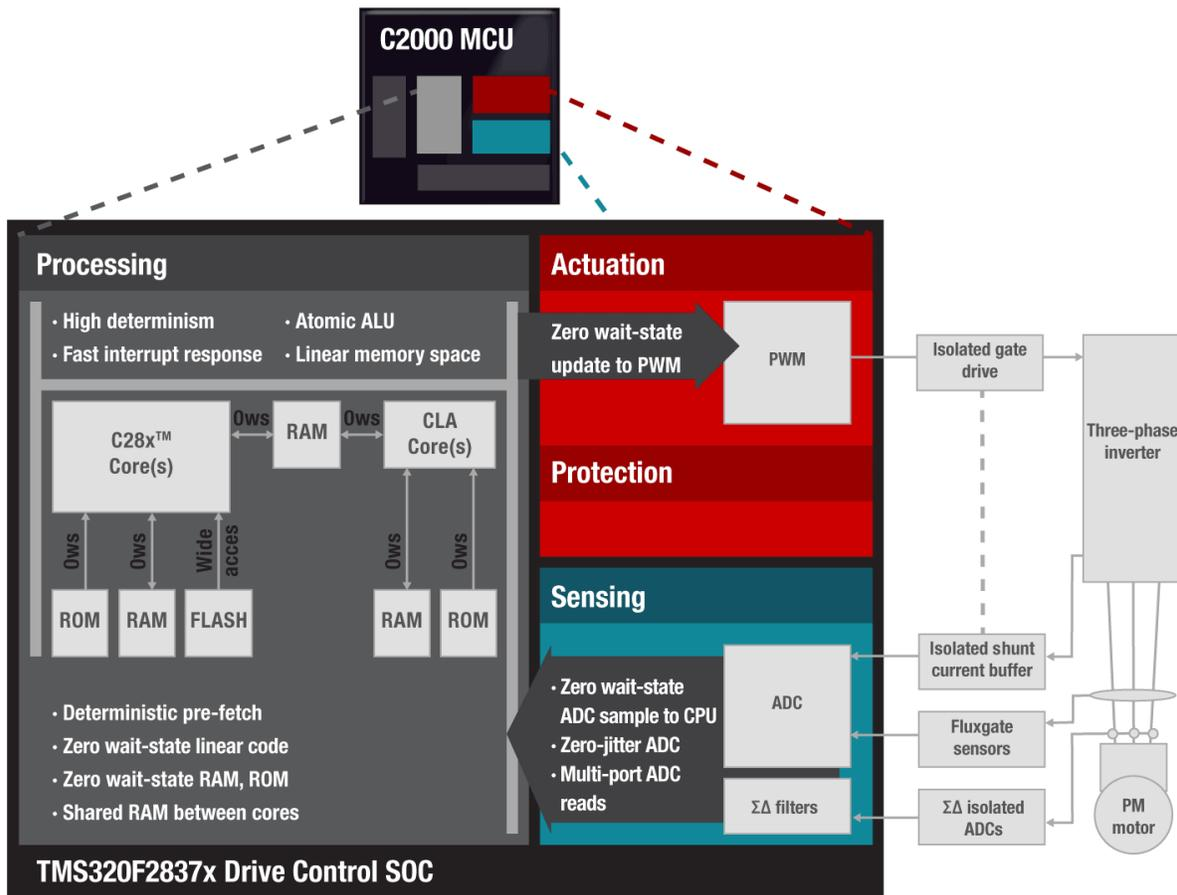
Figure 3. C2000 MCU architecture for real-time motor control
