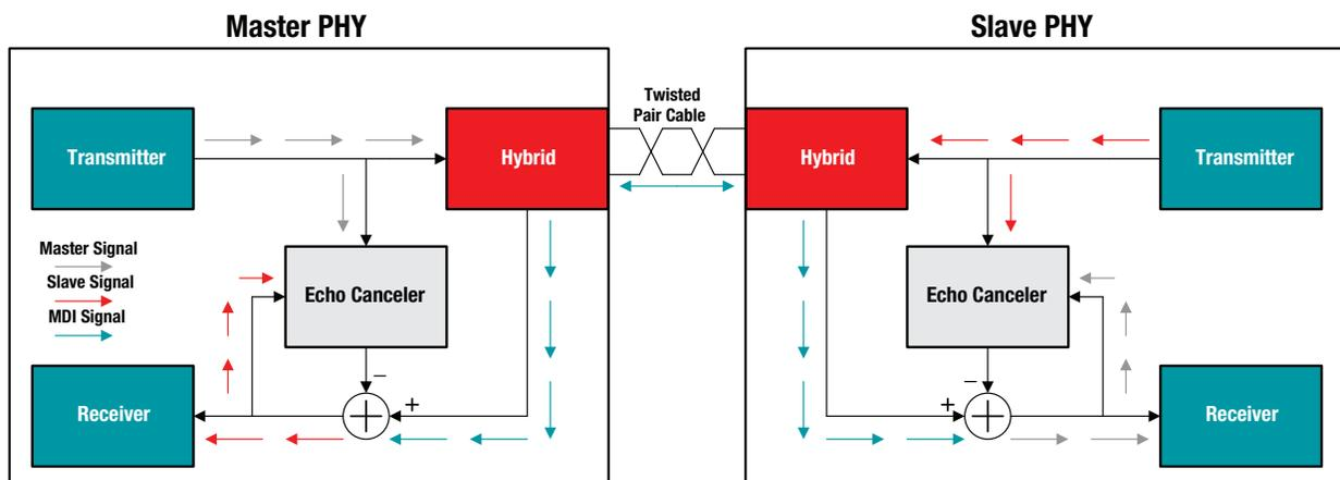
Figure 4. Echo cancellation and hybrid block diagram [11].
