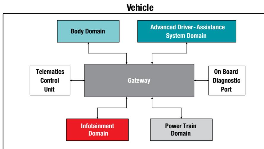
**Figure 1.** Gateway block diagram.
