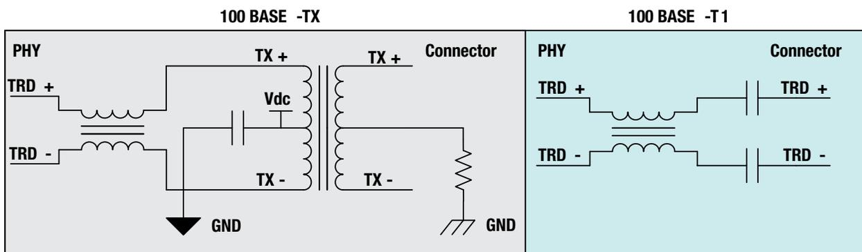
Figure 5. 100BASE-TX vs. 100BASE-T1 DC isolation.
