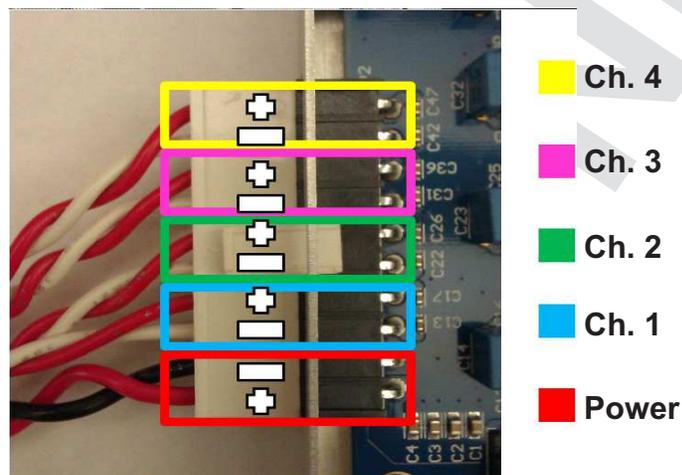
**Figure 4. Power and Speaker Connections to the EVM**
