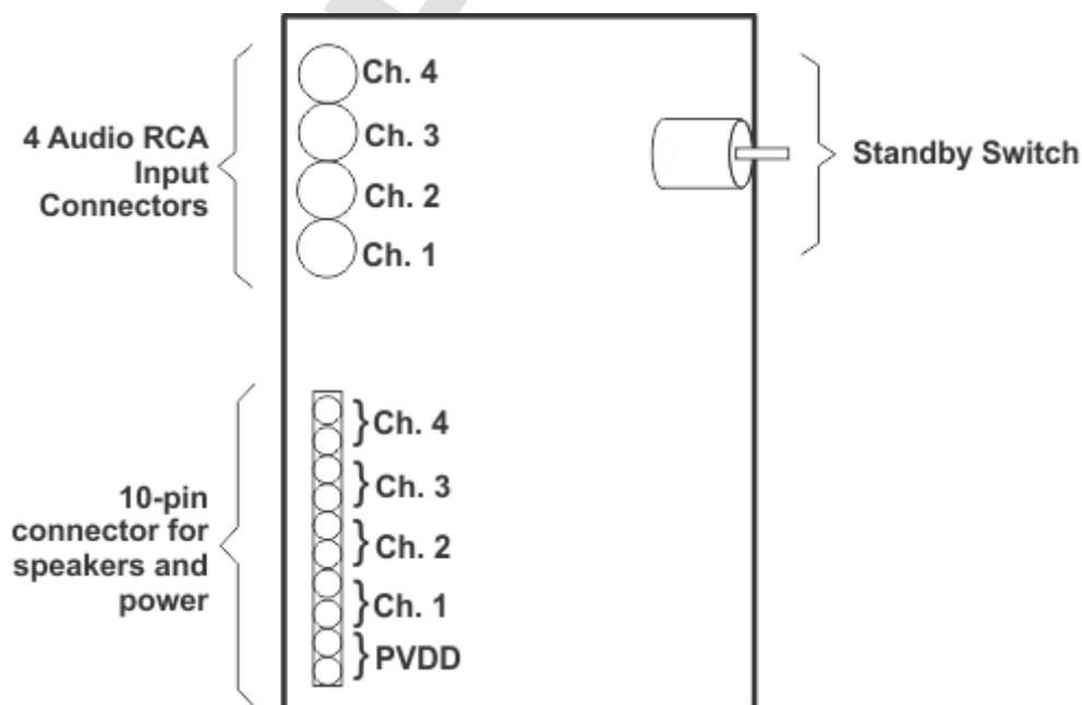
**Figure 1. Connections for Input, Speaker Loads, and Power**
