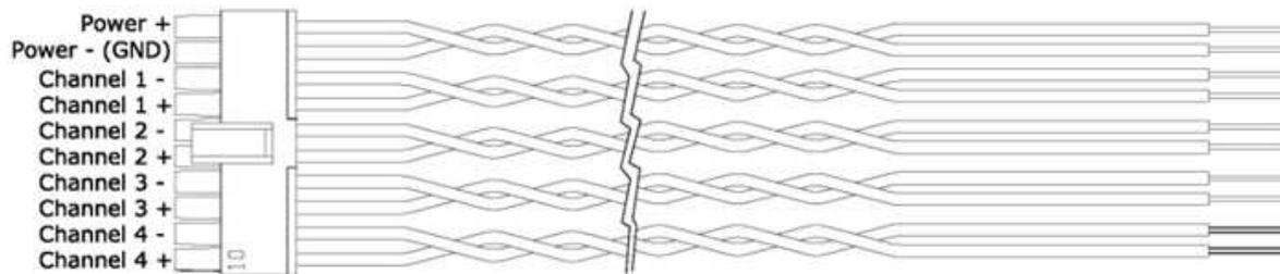
**Figure 3. Wiring Harness for Power and Speaker Connections**
