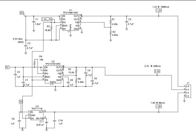
Figure 1. PMP4999 Reference Design Schematic
