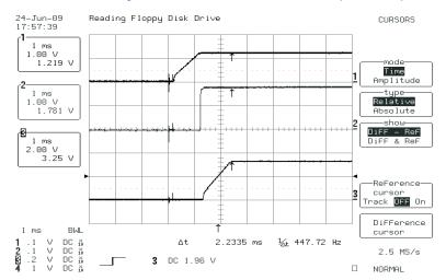
Figure 2. Shows Sequencing in Start up Waveform
